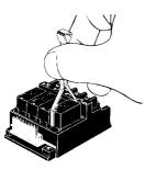
Be sure to turn OFF the power to the Unit before replacing a Relay. Relays must be inserted straight onto the socket connector pins to ensure proper connection.
