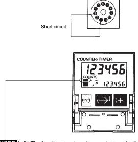
MODE is lit. The function, input mode, or output mode display will be blinking. (The Power OFF display will stop blinking when power comes ON.)
