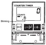
Disconnect terminals 1 and 3 before setting values. When terminals 1 and 3 are disconnected, the "MODE" display will turn OFF and output mode "N" will stop blinking.
