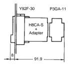
When mounting two or more counters in a vertical line, arrange all the adapters so that the molded springs of the Y92F-30 adapters are positioned on the right and left sides.
