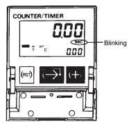
Press the key. "sec" will stop blinking and one of the output modes will begin blinking. The INPUT MODE will automatically enter "T".
