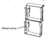
When mounting two or more counters in a horizontal line, arrange all the adapters so that the molded springs of the Y92F-30 adapters are positioned on the top and bottom sides.
