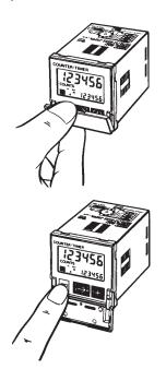
Terminals 1 and 3 must be connected to select timer or counter function using the + key.
