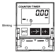
Disconnect terminals 1 and 3 before setting values. When terminals 1 and 3 are disconnected, the "MODE" display will turn OFF and output mode "N" will stop blinking.
