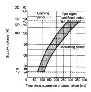
When a power failure occurs, there is a period during which the counter does not respond to the input signal, as shown below, because of lag in the rise in the internal circuit voltage.
