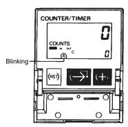
Press the key. "A" will stop blinking and one of the output modes will begin blinking.
