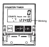
To complete presetting, press the wey so that no place on the display is blinking.
