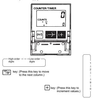
Press the key until the desired digit begins blinking.
