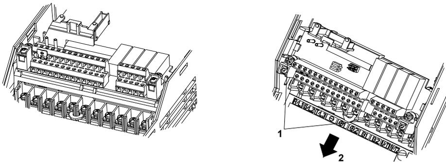
Fig 8.3 Removing the Control Circuit Terminal Card
