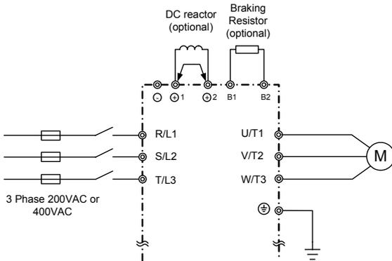
Be sure to remove the short-circuit bar before connecting the DC reactor.
