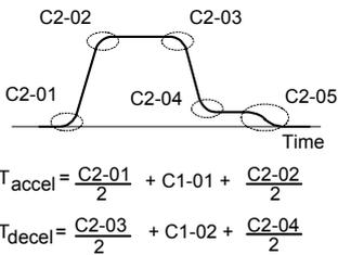
$T_{\text{accel}} = \frac{C2-01}{2} + C1-01 + \frac{C2-02}{2}$ $T_{\text{decel}} = \frac{C2-03}{2} + C1-02 + \frac{C2-04}{2}$ | 0.00 to 2.50  | 0.50 s          | No                      | Q               | Q                | Q                  | Q                       | 20BH              | 6-22 |      |
