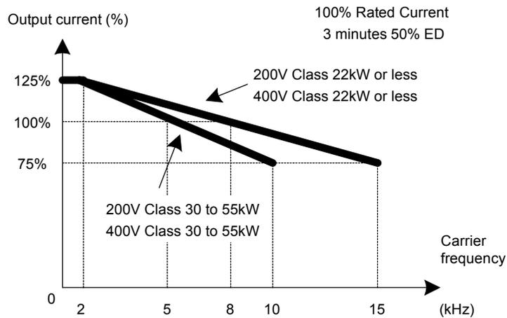
Fig 9.2 Carrier Frequency Derating
