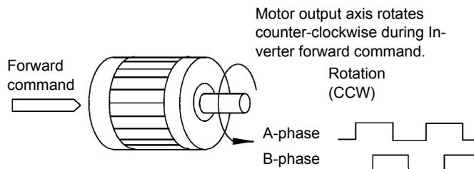
The A-phase leads (CCW) when motor rotation is forward.
