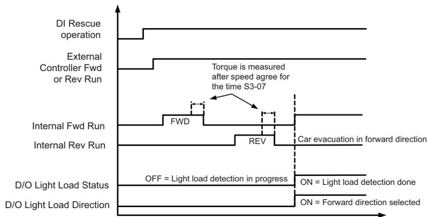
Fig 6.25 Light Load Direction Sequence - FWD is Light Direction
