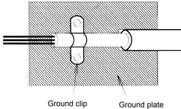
The grounding surfaces must be highly conductive bare metal. Remove any coats of varnish and paint.
