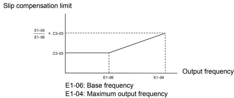
Fig 6.9 Slip Compensation Limit
