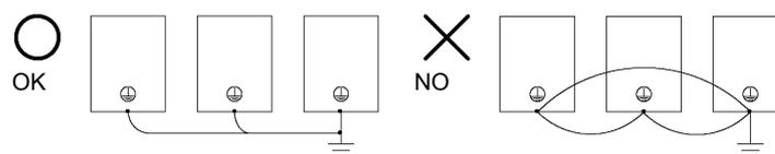
Fig 2.6 Ground Wiring
