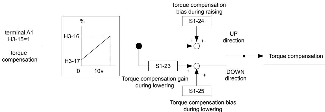
The torque compensation input source can be selected as follows:
