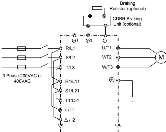
Control power is supplied internally from the DC bus at all inverter models.
