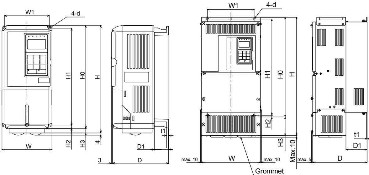
200 V/400 V Class Inverters of 3.7 to 18.5 kW
