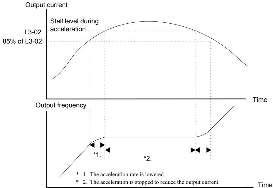
Fig 6.8 Time Chart for Stall Prevention During Acceleration
