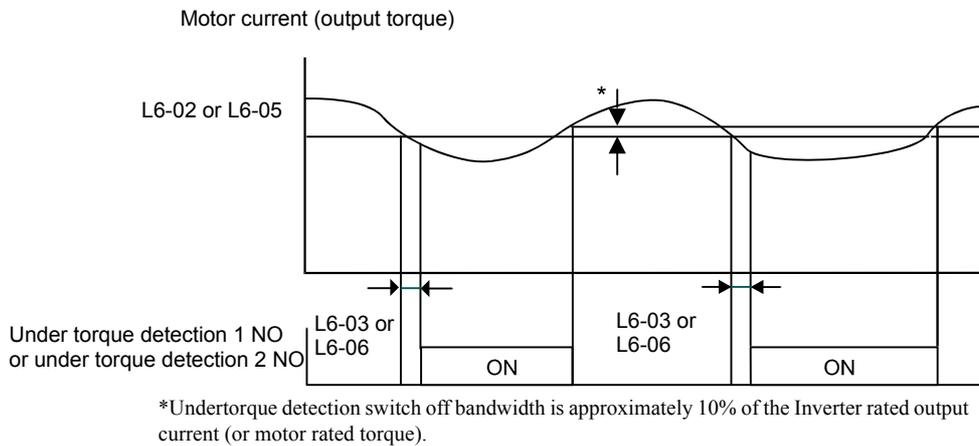
Fig 6.16 Undertorque Detection
