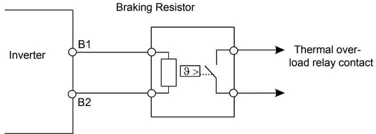
**200 V and 400 V Class Inverters with 22 kW or higher Output Capacity**
