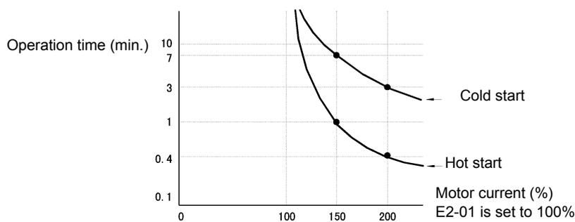
Fig 6.19 Motor Protection Operation Time
