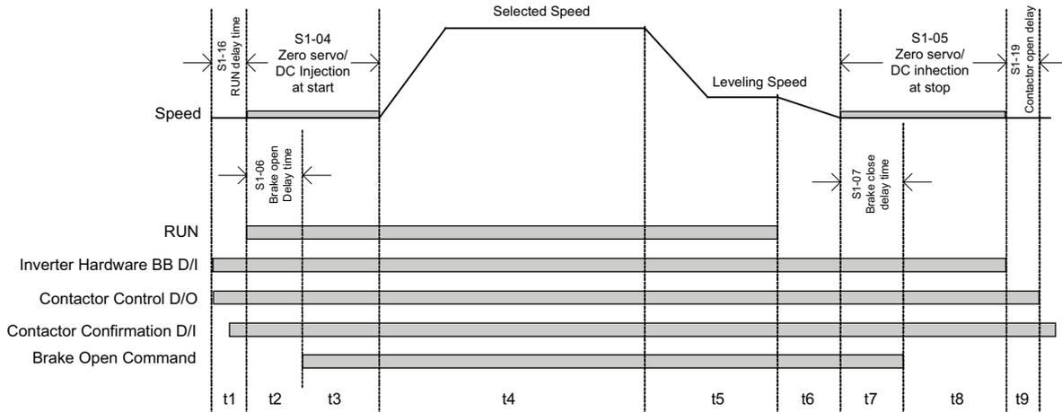
Fig 6.2 Timing chart of Brake sequence without torque compensation at start
