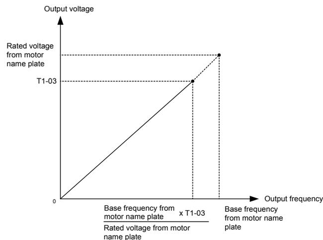
Fig 4.5 Motor Base Frequency and Inverter Input Voltage Setting
