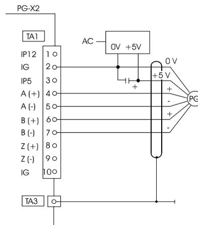
Fig 2.18 PG-X2 Wiring Using a 5 V External Power Supply
