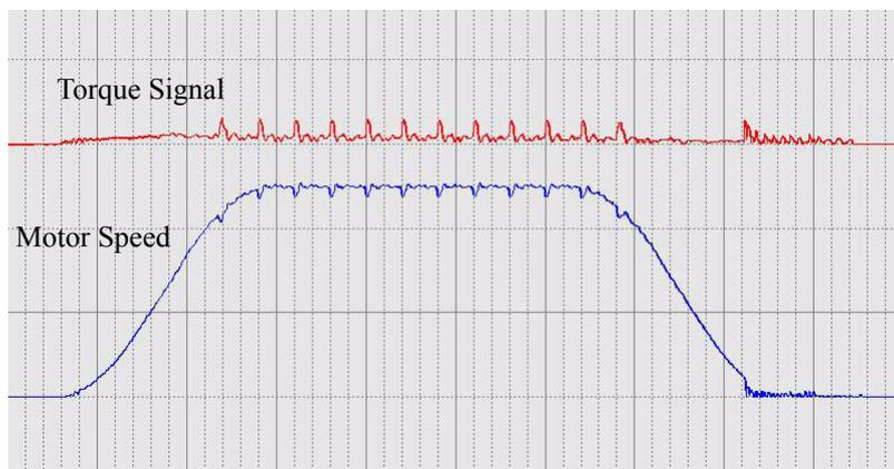
Fig 6.13 Oscillations caused by bad A/D conversion adjustment
