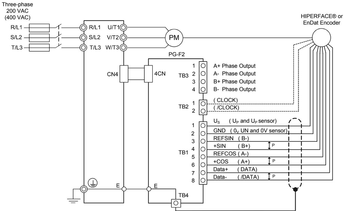
Fig 2.20 PG-F2 Wiring (EnDat signal names in brackets)
