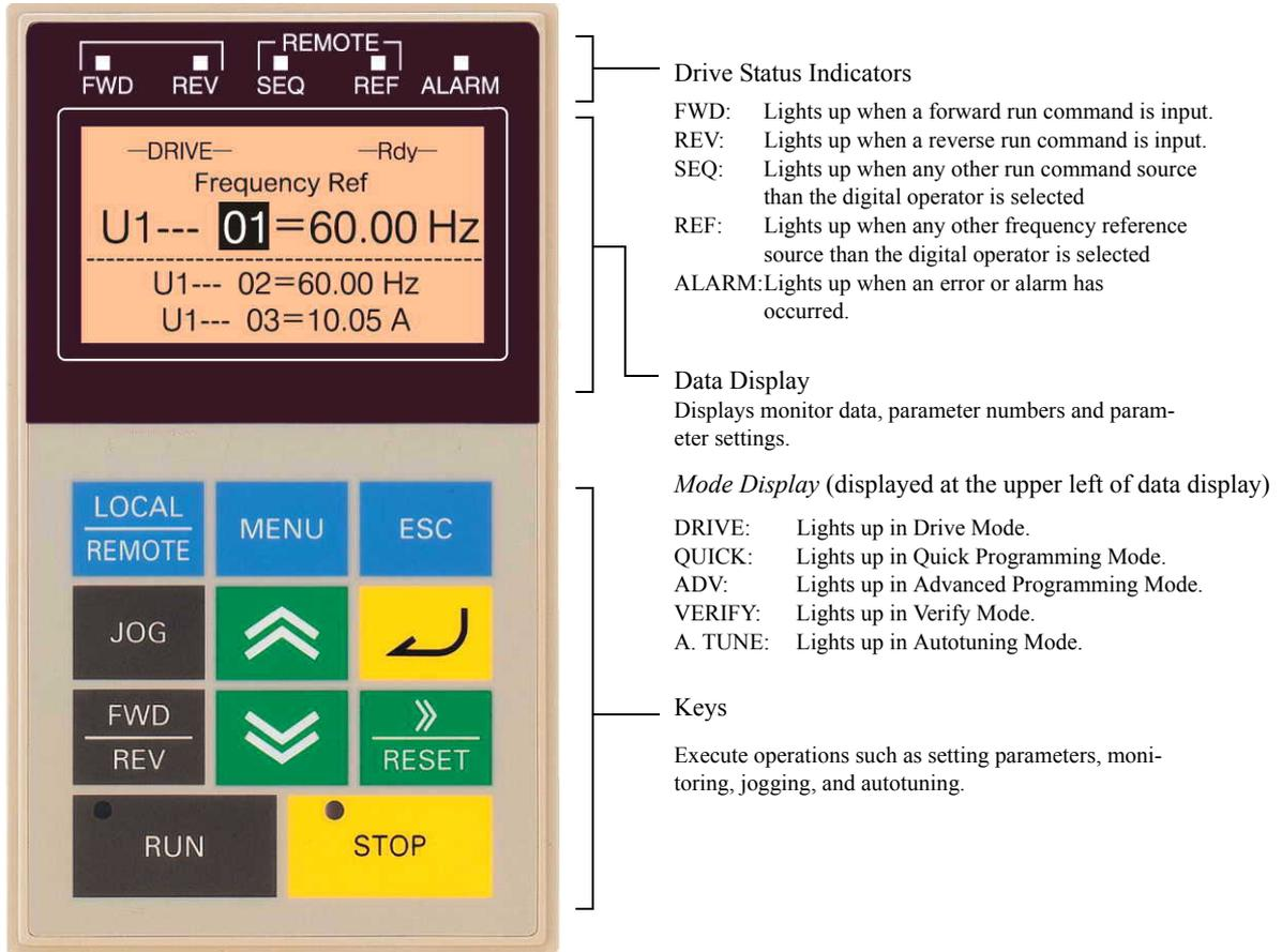
Fig 3.2 Digital Operator Component Names and Functions
