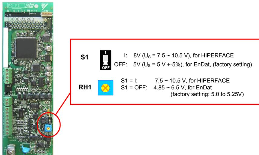
Fig 2.19 PG-F2 Encoder Power Supply Voltage Selection
