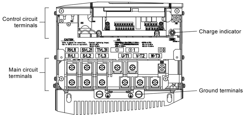
Fig 1.7 Terminal Arrangement (22 kW or More)
