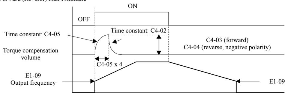
Fig 6.10 Time Chart for Starting Torque Frequency
