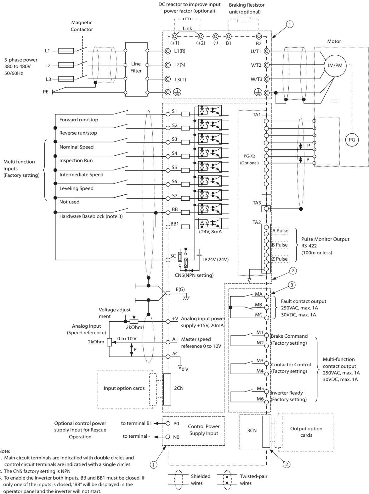
Fig 2.1 Connection Diagram (Model CIMR-L7Z43P7 Shown Above)
