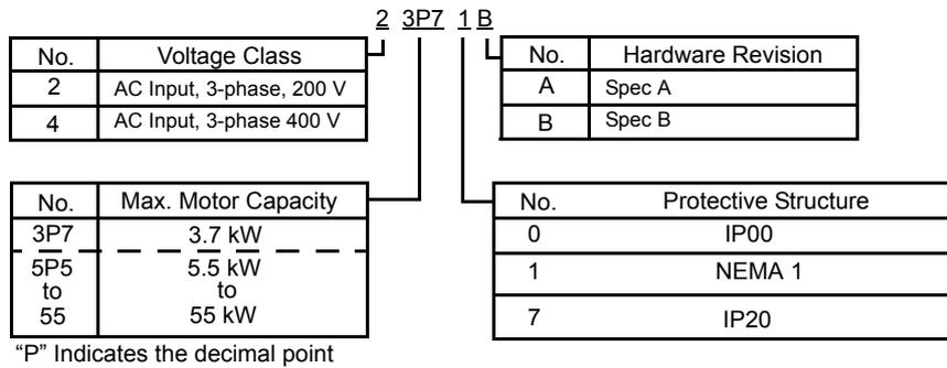
Fig 1.3 Inverter Specifications
