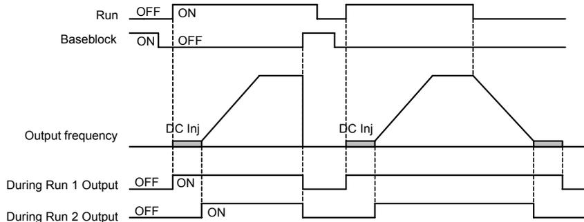
Fig 6.22 Timing Chart for "During RUN" Output
