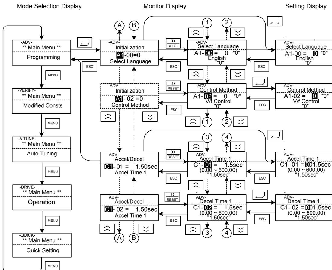
Fig 3.7 Operations in Advanced Programming Mode
