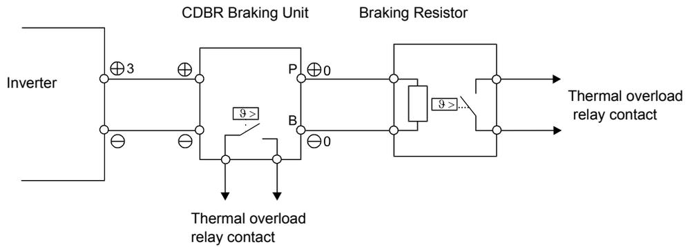
Fig 2.7 Connecting the Braking Resistor and Braking Unit
