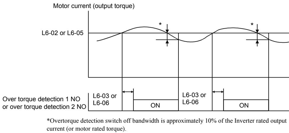
Fig 6.15 Overtorque Detection
