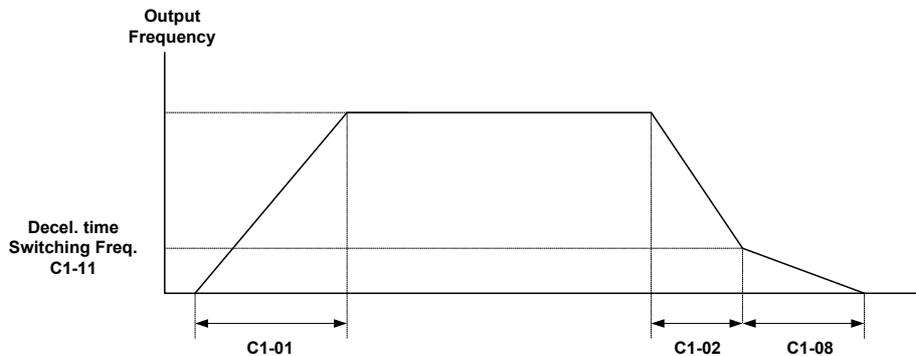
When output frequency  $\geq$  C1-11 the deceleration time 1 (C1-02) is used.
