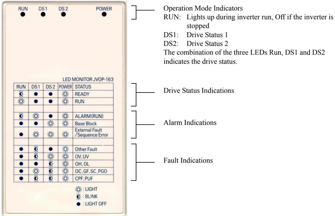
Fig 3.1 Digital Operator Component Names and Functions
