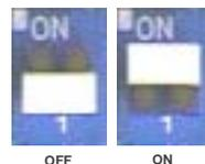
Figure D.3 – PROFIBUS-DP Option Termination Settings
