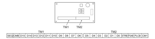
The standard terminal connection of the 3G3AX-DI is shown below.
