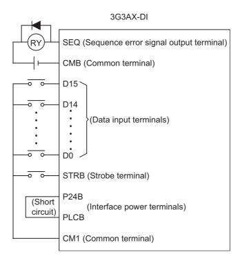
Power is supplied to the input terminals (D0 to D15, STRB) when short-circuiting the P24B and PLCB terminals for the sink logic interface, and short-circuiting the CM1 and PLCB terminals for the source logic interface.
