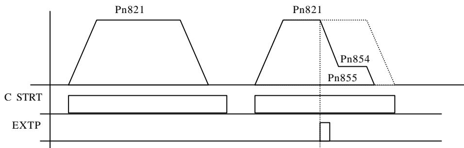
The acceleration and deceleration ramps are defined in parameters Pn822 to Pn826, Pn829, and Pn840 to Pn843.
