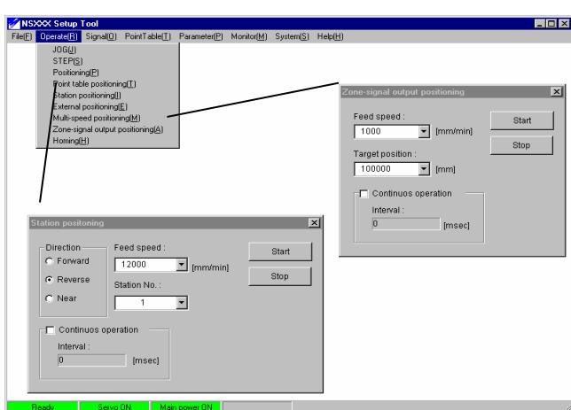
**ZONE-SIGNAL OUTPUT POSITIONING:** Command that executes a positioning with a specified speed and target position. The NOTCH signal will activate if the actual position is inside some position zones.
