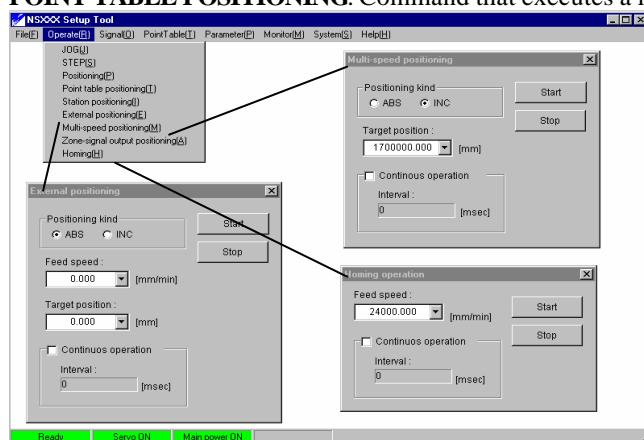
**MULTI-SPEED POSITIONING:** Command that executes a positioning movement to a fixed point where speed change depending of the present position. Both position and speeds are fixed by parameters.
