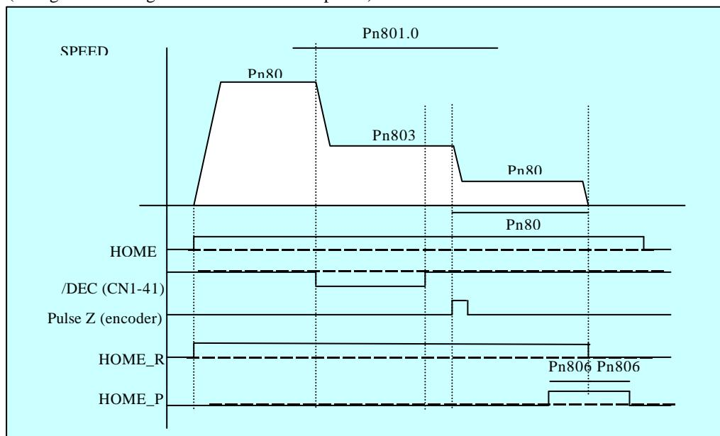
When the HOME command turns on, the origin search starts in the selected direction (Pn801.0) at the origin search speed Pn802. When the rising edge of /DEC signal (CN1-41) comes, the speed decrease to the origin approach speed Pn803 and in the first pulse of Z phase after the falling edge of the /DEC signal the servomotor moves according the selected position in Pn805 (Zero point return final travel distance) at the zero point return creep speed Pn804.
