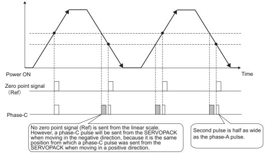
Machine position (Positive direction)
