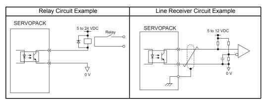
Note: The maximum allowable voltage and current capacities for photocoupler output circuits are as follows.
