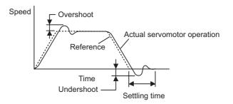
The mode switch function automatically switches the speed control mode between PI control mode and P control mode based on a comparison between the servo's internal value and a user-set detection level shown in *(1) Related Parameters.*
