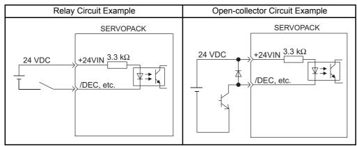
Note: The external power supply (24 VDC) needs the capacity of 50 mA and more.
