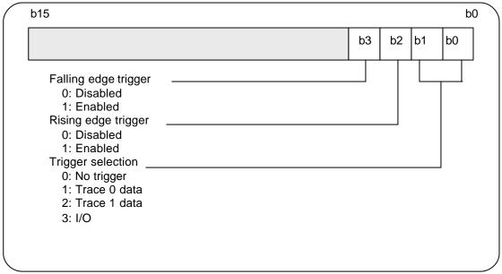
If falling and rising edges are both enabled, the trigger is detected when the data is changed from its previous value. If they are both disabled, it is regarded as "no trigger."
