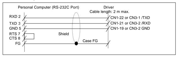
Depending on the personal computer, some communications may not function properly when connected directly to CN1. In that case, use an RS-232C/RS-422A converter.
