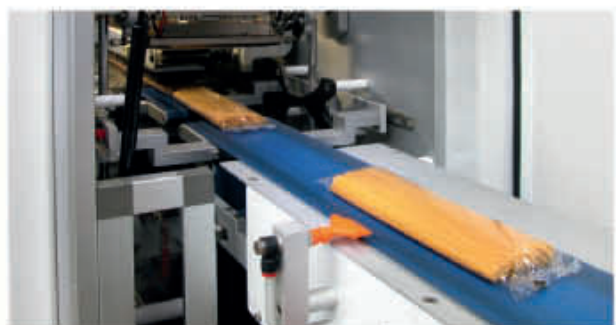
Flow pack machine controlled by Trajexia
