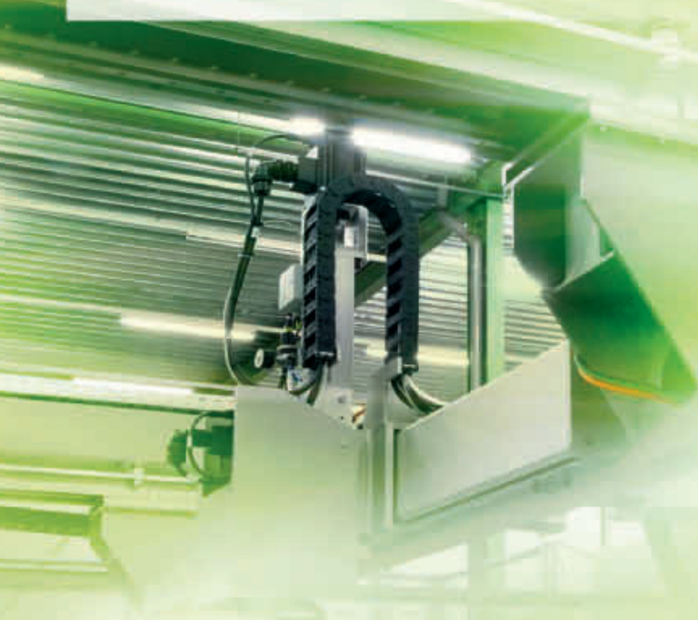
Delta-2 Robot – Pick & Place controlled by Trajexia
