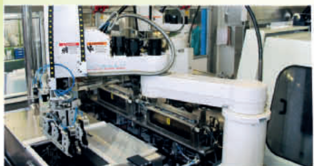
Pick & place with 2 SCARA robots
