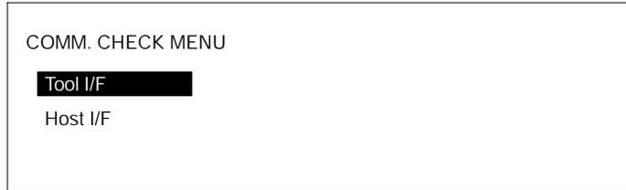
If you select Communications Check, the Communications Check Menu will be displayed. Use the Up and Down Keys to move the bar cursor to the item you want to check, and then press the Enter Key.
