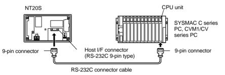
The following are the recommended cables (manufactured by OMRON).
