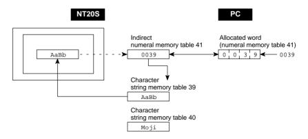
**Reference:** This method is convenient when switching the display at the same location, for example when monitoring a series of words, or when using unique codes to specify individual character strings, etc.
