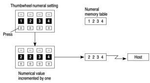
Numerical values cannot be set in thumbwheel type numeral setting fields by using numeric keys.
