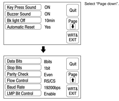
➡ The selected option displayed when the corresponding touch switch is pressed: the options for each switch are indicated below:
