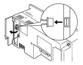
2. Pull out the T-shaped backlight loading tool and replace the backlight.
