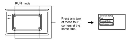
Note that the touch switches used to call the System Menu are not displayed on the screen. If a touch switch displayed in a corner is pressed first, the touch switch will function and the System Menu will not be displayed. To successfully call the System Menu, first press a corner where no touch key is displayed, and then, press any other corner regardless of the presence of a touch key.
