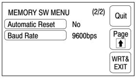
Each time the "Automatic Reset" touch switch is pressed, the setting option "Yes" alternates with "No".
