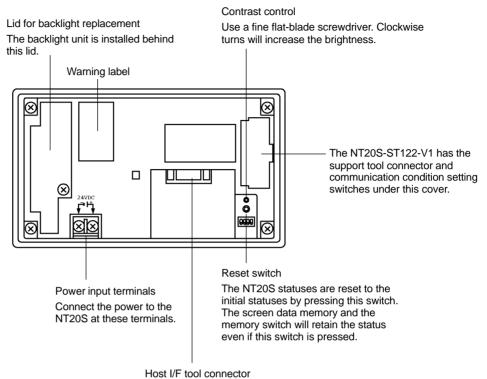
Connect the cable here from a PC/Host or support tool. (On the NT20S-ST122-V1 this connector is for connection to a host only.)
