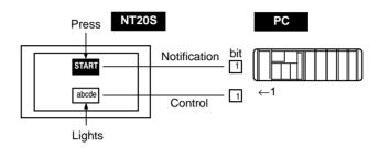
In order to notify the status of a touch switch to the PC, the touch switch must be allocated to a specified PC bit so that it can be managed. Designate the area and bit number.
