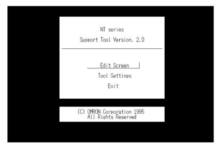
Select "Tool Settings" in the Main Menu to display the "Tool Settings" screen. Settings of PT setting, memory size, and direct setting are made in this screen. Refer to "Setting the support tool for use with the NT20S" on the previous page.
