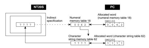
In indirect specification, the contents (numerical value) of the specified numeral memory table are regarded as a memory table number and the contents of the table with this number are displayed.
