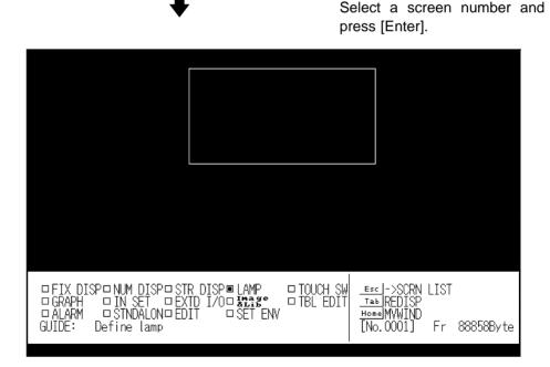
Create screen data in the Edit screen. Data of one screen can be created by registering (laying out) the following display elements and attributes on the screen.
