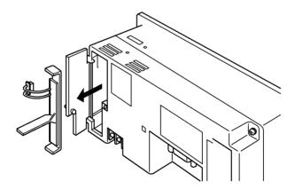
Re-install the backlight and connect its connector to the NT20S.
