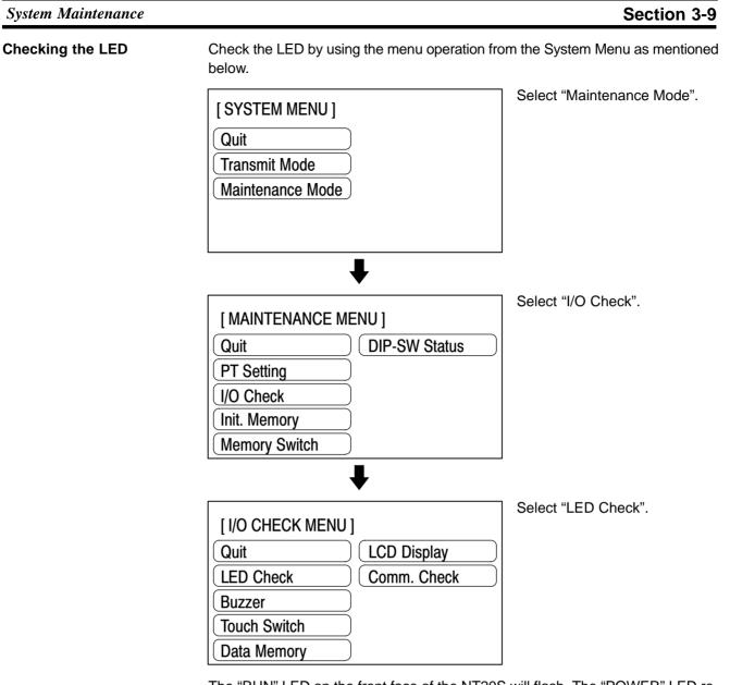
The "RUN" LED on the front face of the NT20S will flash. The "POWER" LED remains lit.
