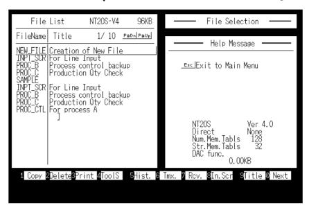
Select a file used for storing the screen data for the NT20S in the "File List" screen.
