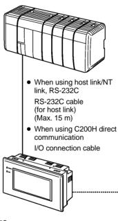
NT20S Gives displays of production line monitoring and instructions to the operation site and notifies the switch ON/OFF status and numeric value inputs to the Host. Host (PC manufactured by OMRON, personal computer, etc.) Controls NT20S as required while controlling machines and monitoring the production line. Host link: C series, CQM1, CVM1/CV series PC, C H, CQM1,
