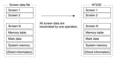
When the screen data is transmitted from the support tool to the NT20S, the screen data already existing in the NT20S will be erased.
