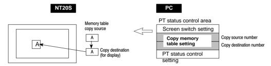
Write a memory table number etc. to the copy memory table setting area in the PT status control area in the PC memory. Data will be copied between the memory tables in the NT20S and the displayed value will change accordingly.
