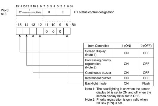
The PC status control bits remain unchanged if the NT20S status is changed with the screen attributes or memory switches, which means that the statuses of the PT status control bits do not match the actual status of the NT20S. For example, the buzzer may sound even though the setting for continuous buzzer bit 13 is "OFF".
