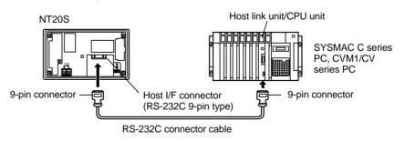
**Note:** The connector cable wiring for the C series CPU unit (C□□H) is different from that for the other PCs. For details, refer to Appendix G Method for Making the Cable for Connection to the Host (page 256).
