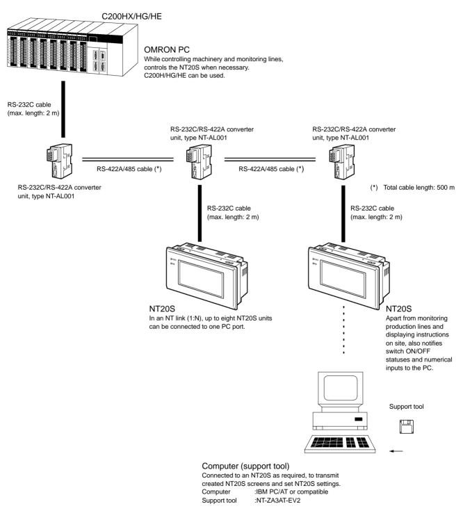
**Reference:** When connecting the C200HX/HG/HE and an RS-232C/RS-422A converter unit, use a converter unit whose lot number is 15Y5 or later. Converter units of lot numbers previous to 15Y5 cannot be connected.
