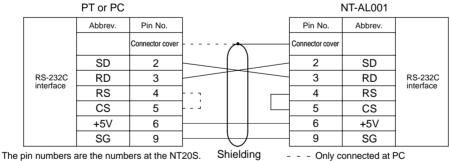
For the pin numbers at the PC, refer to the manual Wire for the PC used.
