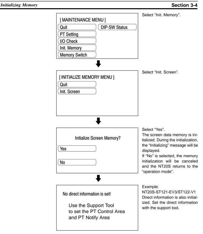
After initialization of the screen data memory, the system enters the operation mode. At this point, nothing is displayed on the screen of the NT20S. Return to the System Menu, select the Transmit Mode, and transmit the screen data from the support tool.
