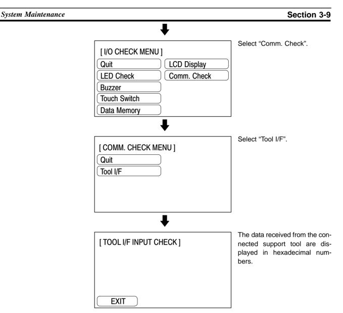
When the check is finished, press the Exit touch switch. The NT20S will enter the I/O CHECK MENU.
