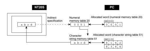
This specification method is a little complex, but it allows the display to be changed more easily according to the circumstances. In the example above, if 1 were added to the contents of memory table 20 to give 52, the contents of memory table 52 would be displayed instead.
