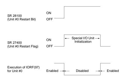
While the Restart Flag (SR 27400) is ON, normal END refreshing is performed and the Special I/O Unit is initialized. This processing occurs regardless of the settings in DM 6620, DM 6621, and DM 6623, which relate to Special I/O Unit refreshing. IORF(97) instructions in the program won't be executed for the initializing Unit until initialization is completed.
