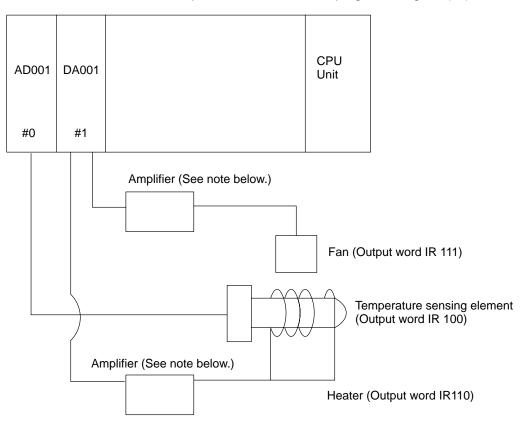
**Note** Motors and heaters cannot be directly connected from an Analog Output Unit. An amplifier (i.e., a current amplification circuit) is required.
