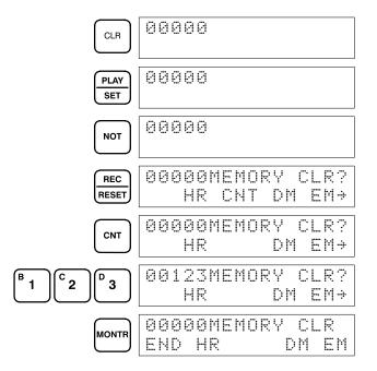
Clearing Selected EM Banks When a partial memory clear operation is being performed, specific banks can be selected for clearing rather than selecting the entire EM area. In the following example, EM banks 0 and 2 are selected for clearing.
