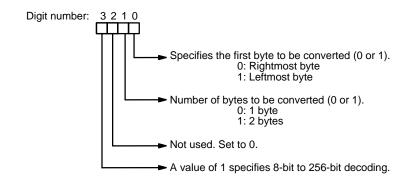
The 4 possible C values and the conversions that they produce are shown below. (In S, 0 indicates the rightmost byte and 1 indicates the leftmost byte.)
