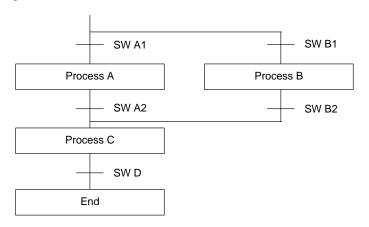
The program for this process, shown below, starts with two SNXT(09) instructions that start processes A and B. Because of the way 00001 (SW A1) and 00002 (SB B1) are programmed, only one of these will be executed to start either process A or process B. Both of the steps for these processes end with a SNXT(09) that starts the step for process C.
