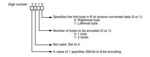
Three possible C values and the conversions that they produce are shown below. (In R, 0 indicates the rightmost byte and 1 indicates the leftmost byte.)
