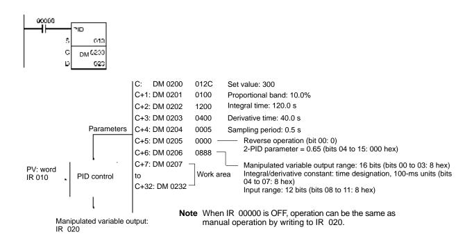
Input Values and Manipulated Variable Ranges The number of valid input data bits for the measured value is designated by the input range setting in C+6, bits 08 to 11, and the number of valid output data bits for the manipulated variable output is designated by the output range setting in C+6, bits 0 to 3. These ranges are shown in the following table.
