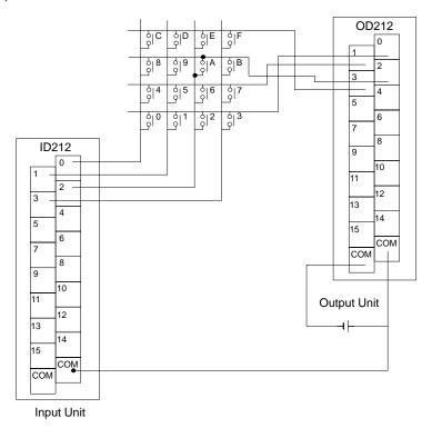
The inputs connected to the input terminals must be on a DC Input Unit with 8 or more input points and the outputs connected to the output terminals must be from a Transistor Output Unit with 8 points or more.
