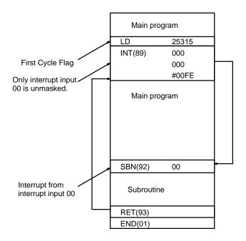
**Note** Depending on the setting of DM 6621 in the PC Setup, Host Link servicing, Remote I/O servicing, Special I/O Unit servicing, and individual instruction execution will be completed before the subroutine is executed. Refer to page 282 for details.
