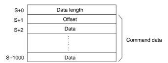
The data length, offset, and command data settings depend on the process number that is specified, as shown in the following table.
