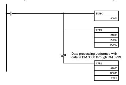
**Note** If BXF2(—) were used to perform the data transfers, any EM bank could be specified and EMBC(—) would not be required to select EM bank 1.
