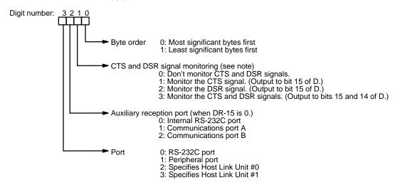
Note Data is not output when the CTS and DSR signals are monitored.
