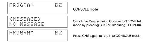
Expansion TERMINAL Mode The Programming Console can be put into Expansion TERMINAL mode by turning ON AR 0709. Pin 6 of the CPU Unit's DIP switch must be ON.
