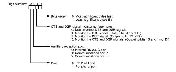
Note Data is not output when the CTS and DSR signals are monitored.
