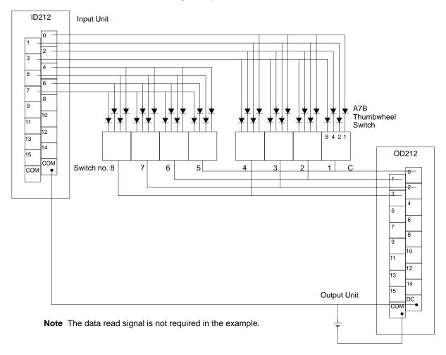
The inputs must be connected to a DC Input Unit with 8 or more input points and the outputs must be connected from a Transistor Output Unit with 8 or more output points.
