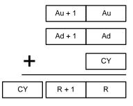
ADBL(—) can also be used to add signed binary data. The overflow and underflow flags (SR 25404 and SR 25405) indicate whether the result has exceeded the lower or upper limits of the 32-bit signed binary data range. Refer to page 27 for details on signed binary data.
