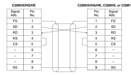
**Note** Ground the FG terminal of the PC to a resistance of 100  $\Omega$  or less.
