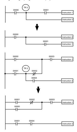
Note TR bits are only used when programming using mnemonic code. They are not necessary when inputting ladder diagrams directly. The above limitations on the number of branching points requiring TR bits, and considerations on methods to reduce the number of programming instructions, still hold.
