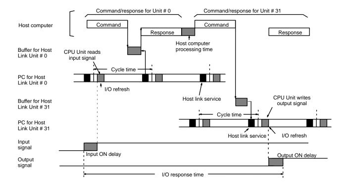
The equations used to calculate the minimum and maximum cycle times are given below. The number of cycles required for each PC depends on the amount of data being read/written.
