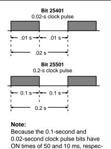
tively, the CPU Unit may not be able to accurately read the pulses
