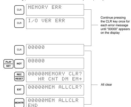
The following procedure is used to clear memory completely.
