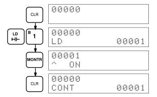
**Note** The status of TR bits SR flags SR 25503 to 25507 (e.g., the arithmetic flags), cleared when END(01) is executed, cannot be monitored.
