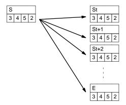
BSET(71) can be used to change timer/counter PV. (This cannot be done with MOV(21) or MVN(22).) BSET(71) can also be used to clear sections of a data area, i.e., the DM area, to prepare for executing other instructions.
