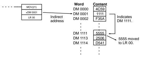
When using indirect addressing, the address of the desired word must be in BCD and it must specify a word within the DM area. In the above example, the content of \*DM 0000 would have to be in BCD between 0000 and 6655.
