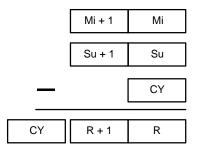
SBBL(—) can also be used to subtract signed binary data. The overflow and underflow flags (SR 25404 and SR 25405) indicate whether the result has exceeded the lower or upper limits of the 32-bit signed binary data range. Refer to page 27 for details on signed binary data.
