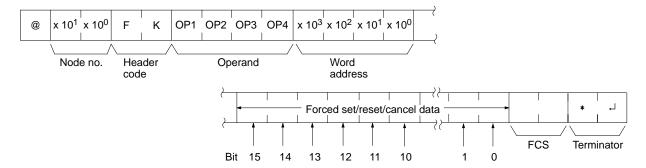
For data areas IR, SR, LR, HR, and AR, the "Operand" parameter indicates the data area where the bit will be force-set and the "Word address" parameter indicates the word address.
