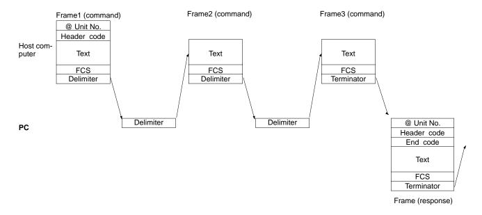
**Using the TXD(—) Instruction** The TXD(—) instruction can be used to transmit data from the PC's data area to the host computer. There is no response from the host computer. The TXD(—) instruction will be executed after the response has been transmitted if TXD(—) is executed while a response to a Host Link command is being returned to the host computer.
