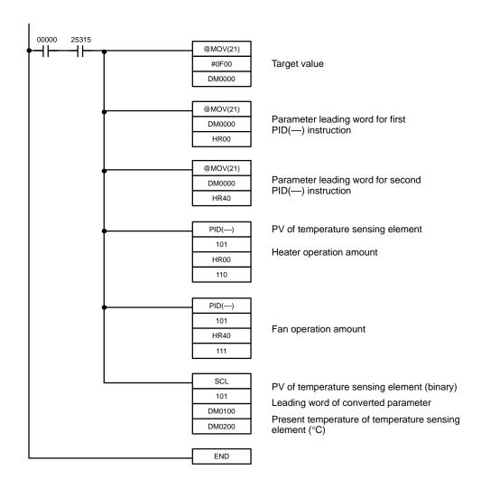
**Note** When using PID(—) or SCL(—), make the data settings in advance with a Peripheral Device such as the Programming Console or SSS.
