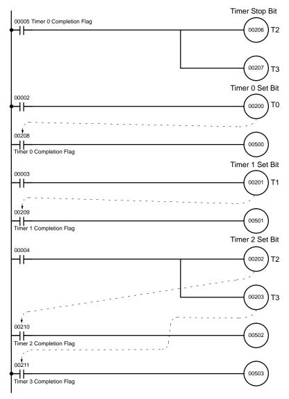
Timers 2 and 3 stop operating when the emergency stop input goes ON.
