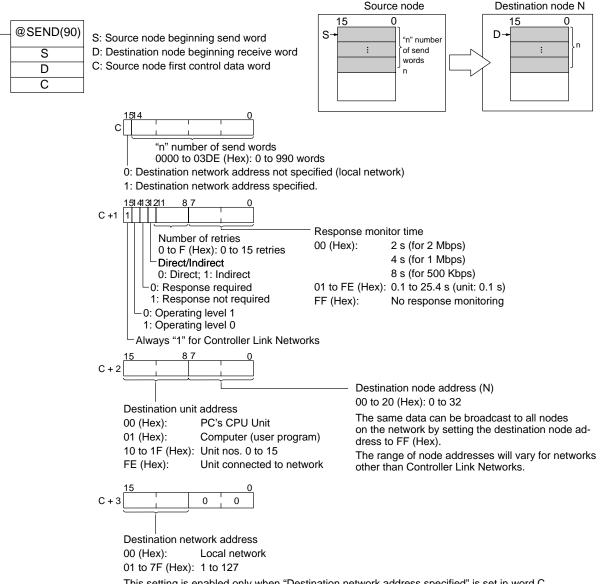
This setting is enabled only when "Destination network address specified" is set in word C. When specifying a destination network address, set all the nodes in the routing tables. For details on routing tables, refer to refer to the section on network interconnections in the *Controller Link Unit Operation Manual (W309)*.
