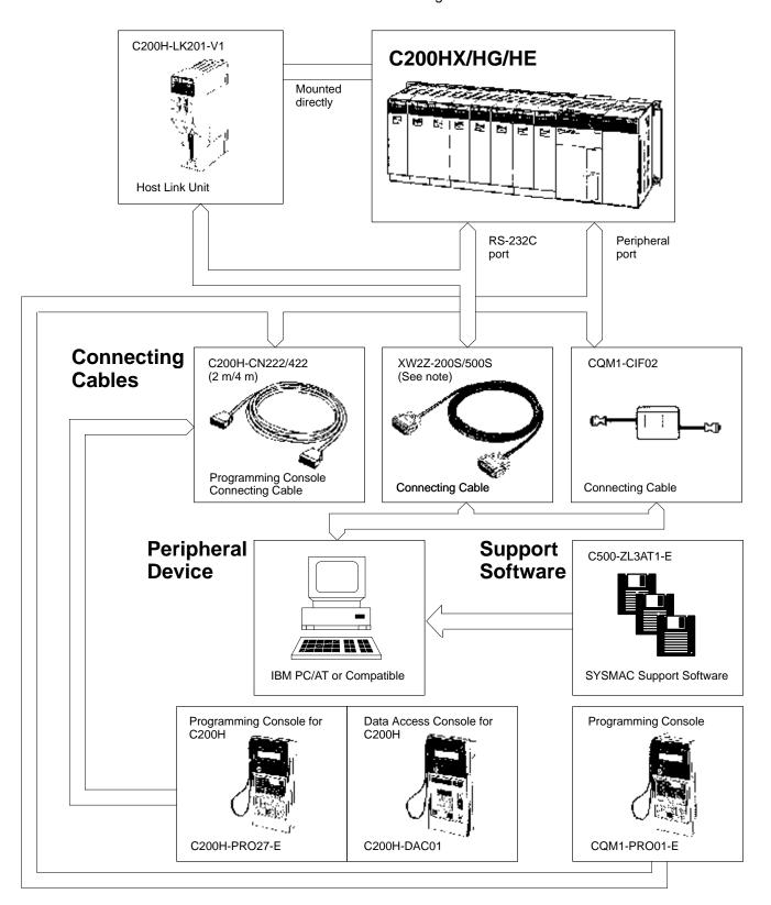
**Note** The connector of the XW2Z-200S/500S Connecting Cable is a male 25-pin terminal. An adapter is required for the 9-pin male D-sub terminal on the IBM PC/AT or compatible side.
