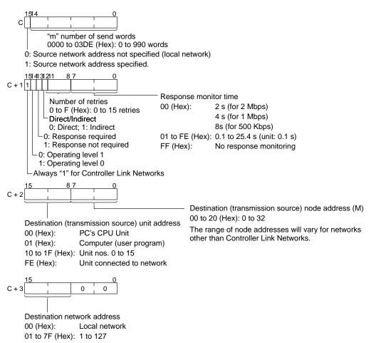
This setting is enabled only when "Destination network address specified" is set in word C. When specifying the destination network address, set all the nodes in the routing tables. For details on the routing tables, refer to the section on network interconnections in the *Controller Link Unit Operation Manual (W309)*.
