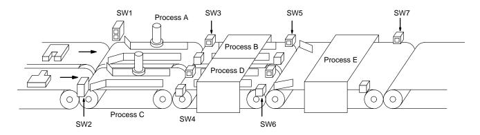
The following diagram demonstrates the flow of processing and the switches that are used for execution control. Here, process A and process C are started together. When process A finishes, process B starts; when process C finishes, process D starts. When both processes B and D have finished, process E starts.
