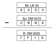
The absolute value of the true result (80E8=33,000) can be obtained by taking the 2's complement of 7F18 using NEG(—).
