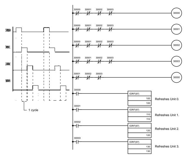
**Note** IR 30000 is used in an OUT instruction twice in this program. Although acceptable in the above example, this type of duplication is not usually allowed unless there is a specific reason and then only when proper operation can be ensured.
