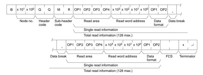
The "Read area" indicates the data area, the "Read word address" indicates the word address, and the "Data format" indicates the bit number (00 to 15) or entire word (CH).
