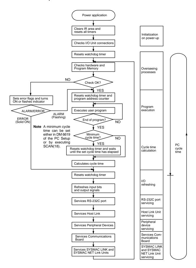
The first three operations immediately after power application are performed only once each time the PC is turned on. The rest of the operations are performed in cyclic fashion.
