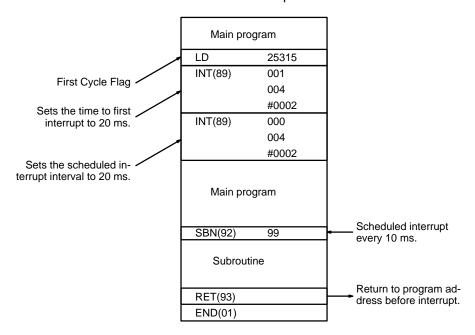
**Note** Depending on the setting of DM 6621 in the PC Setup, Host Link servicing, Remote I/O servicing, Special I/O Unit servicing, and individual instruction execution will be completed before the subroutine is executed. Refer to page 282 for details.
