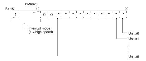
Note Disabling special I/O refreshing in the normal cycle to refresh special I/O in an interrupt subroutine is necessary only in the high-speed mode. Disabling normal cycle refreshing of special I/O during normal interrupt mode will be ignored and the special I/O will be refreshed both in the normal cycle and in the interrupt subroutine.
