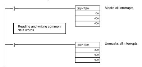
Data concurrence can also be a problem if interrupts occur during data transfers occurring in servicing for Special I/O Units, remote I/O, or Host Link Systems. For any of these, data can be non-concurrent down to byte units.
