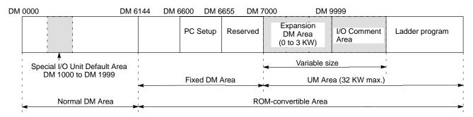
**Note** Refer to the SYSMAC Support Software (SSS) Manual for details on using SSS to allocate UM for expansion DM or I/O comments. Refer to 7-2-15 UM Area Allocation for details on using the Programming Console to allocate UM for expansion DM.
