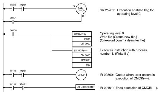
$\,$  DM 0000 to DM 0007 contain the control data and DM 0098 to DM 0199 contain the command data, as shown below.
