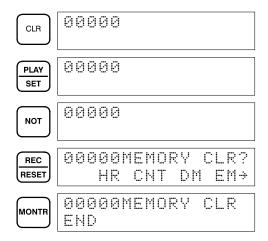
Note When the write-protect switch (pin 1 of the CPU Unit's DIP switch) is set to ON the UM area (from DM 6144 through the ladder program) will not be cleared. Other data areas, such as HR, AR, CNT, and DM from DM 0000 to DM 6143 will be cleared.
