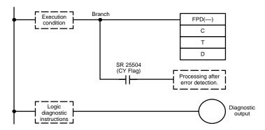
When the execution condition is OFF, FPD(—) is not executed. When the execution condition is ON, FPD(—) monitors the time until the logic diagnostics condition goes ON, turning ON the diagnostic output. If this time exceeds T, the following will occur:
