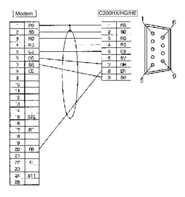
**Note** Ground the FG terminals on the PC and at the other device to 100  $\Omega$  or less. Refer to the *C200HX/HG/HE Installation Manual* and the documentation included with the other device for details.
