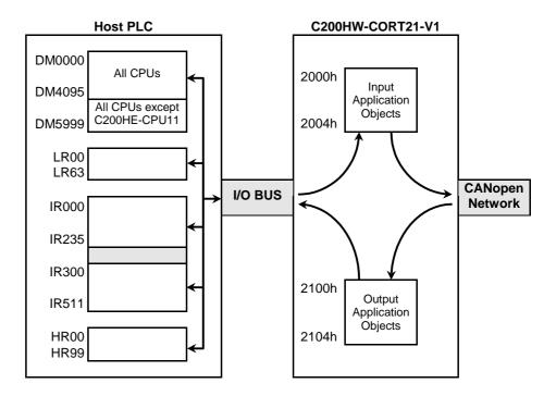
The core of the C200HW-CORT21-V1 is the object dictionary. The Input and Output Application Objects are part of this object dictionary.
