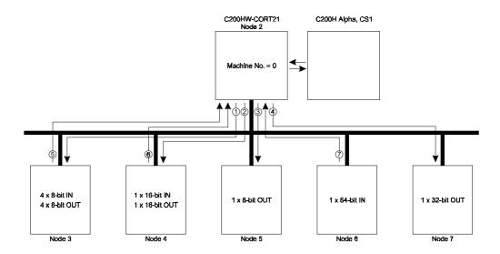
There are in total 7 logical connections to the C200HW-CORT21-V1. From the C200HW-CORT21-V1 point of view, connections 1 to 4 are transmit PDOs and connections 5 to 7 are receive PDOs.
