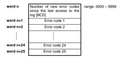
Word n in the message structure indicates how many new errors have occurred since the last time the error log was read. Word n will not count any further than 9999 new errors. Only the 25 most recent errors are stored in the error log.
