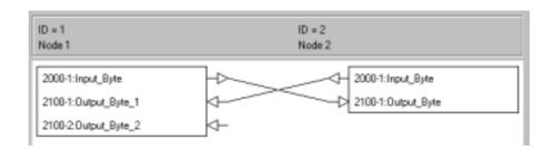
The input byte of Node 1 is linked to the Output byte of Node 2 with two mouse clicks. The Input byte of Node 2 is connected to the first Output byte of Node 1 the same way. The configuration tool will automatically assign an available COB-ID to each connection made. Refer to the manual of a configuration tool for more details.
