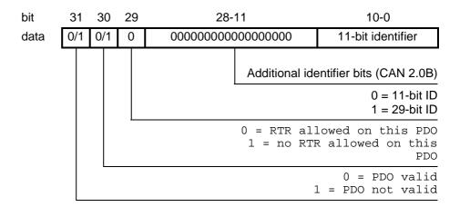
Note: C200HW-CORT21-V1 supports only 11-bit identifiers, and no Remote Transmission Requests (RTR). Therefore all its valid PDOs have COB-ID's with the structure 40000xxxh. For PDO linking, only the identifier (xxx) is relevant.
