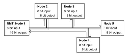
Nodes 2 to 5 are 8 digital input + 8 digital output modules. Node 1 is the Network Management Master, which is also able to transmit and receive data over the network. Note that the terms 'input' and 'output' are with respect to the network.
