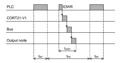
$t_{UDC}$  : The transmission time of a user defined CAN message
