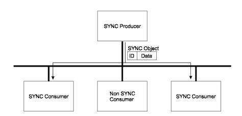
CANopen devices may be SYNC Producer, SYNC Consumer, neither, or both. Specific behaviour as producer or consumer is configurable.
