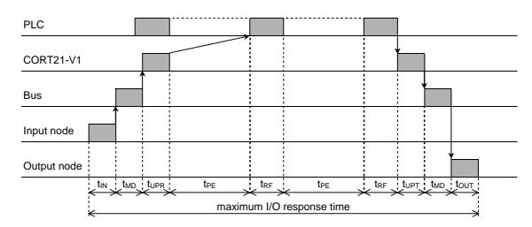
t<sub>IN</sub> : Input Node ON (OFF) delay
