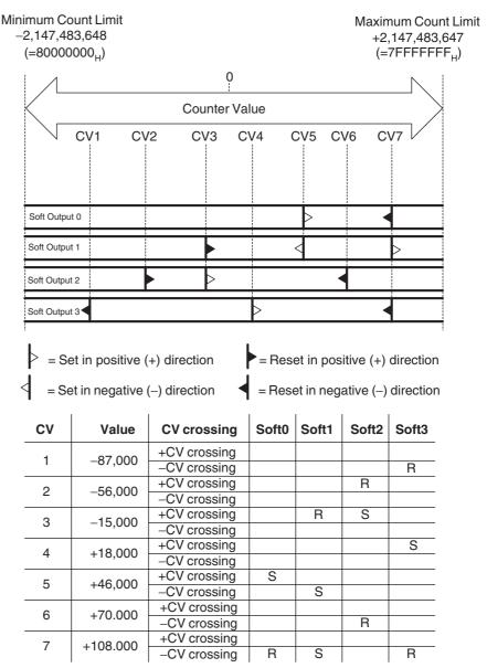
In this example 7 Comparison Values are specified. On reaching a Comparison Value an Output can be Set or Reset depending on the crossing direction. If the
