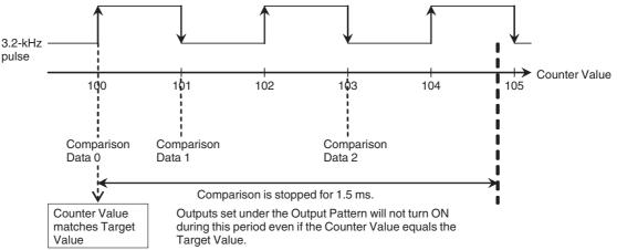
Comparison Stoppage for IOWR- and IORD-instruction Execution Comparison is stopped during the execution of IOWR/IORD-instructions and remains stopped until the processing of the instruction has been completed. The Data Transfer Busy bit is ON during this time.
