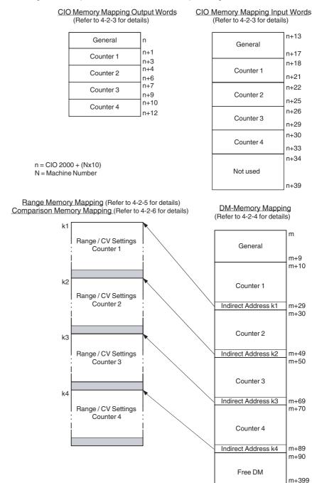
$$\begin{split} m &= D\ 20000 + (Nx100) \\ N &= Machine\ Number \\ k1, k2, k3, k4 &= Any\ available\ address\ in\ DM/EM \\ (Refer to\ 4-2-2\ for\ more\ details\ about\ Indirect\ Addressing) \end{split}$$
