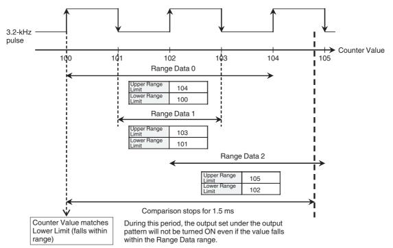
Comparison Stoppage When IOWR and IORD-instructions Executed Comparison is stopped during the execution of IOWR/IORD-instructions and remains stopped until the processing of the instruction has been completed. The Data Transfer Busy bit is ON during this time.
