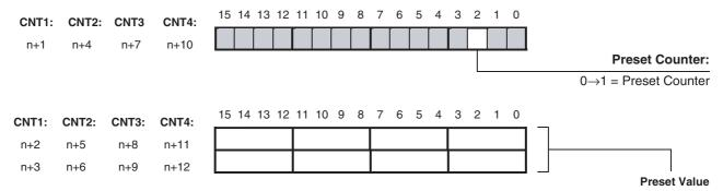
Set between 00000000<sub>H</sub> and FFFFFFF<sub>H</sub> (Circular Counter) Set between 80000000<sub>H</sub> and 7FFFFFF<sub>H</sub> (Linear Counter)
