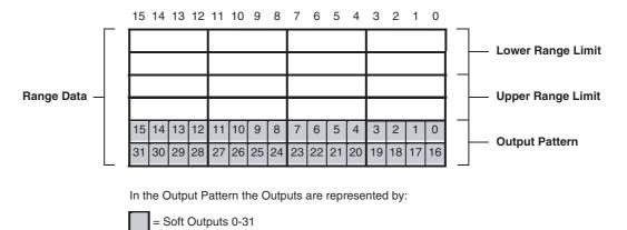
In the Output Pattern of the Range every single Output can be configured to turn ON when that Range is active. To configure an Output to turn ON you must set the corresponding bit to 1. If multiple Ranges of a Counter are active at the same time, the Output Patterns of those Ranges are logically OR'ed to become the Output Pattern of that Counter.
