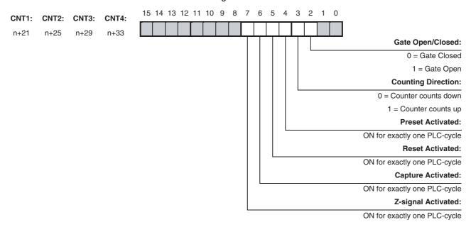
The Reset, Preset, Capture and Z-signal Activated Bits are ON for exactly one PLC-cycle after the occurrence of a (short) pulse which was detected since the previous I/O Refresh.
