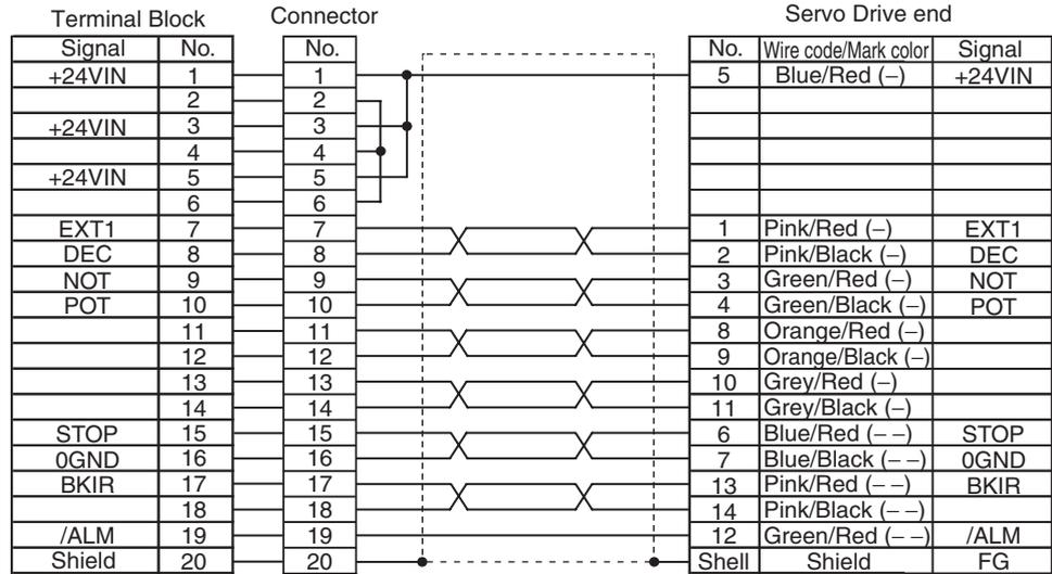
Connector at Connector Terminal Block
