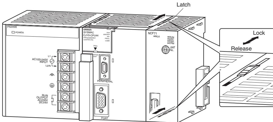
**Note** If the latches are not completely locked, the PCU may not function properly.
