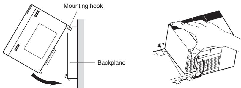
2. Insert the connector on the back of the CPU properly into the connector on the Backplane.
