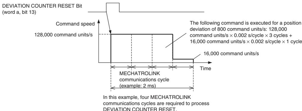
In this example, the movement command to eliminate the position deviation of 800 command units exceeds the movement possible in one MECHATROLINK communications cycle at a speed of 128,000 command units/s, so the command is executed over multiple cycles (four total).
