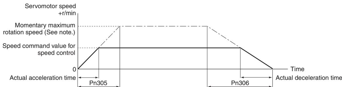
**Note** The momentary maximum rotation speed depends on the Servomotor used. Refer to the momentary maximum rotation speed for the Servomotor used. The following values apply to W-series Servomotors.
