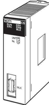
The Position Control Unit is a CS/CJ-series CPU Bus Unit. The Position Control Unit (PCU) receives commands from the CPU Unit's internal Auxiliary Area and outputs positioning commands to MECHATROLINK-II Servo Drives. MECHATROLINK is a registered trademark of MECHATROLINK Members Association.
