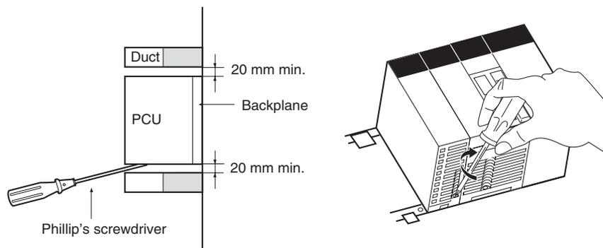
3. Tighten the screw on the bottom of the PCU using a Phillip's screwdriver. When mounting the PCU inside equipment, provide the minimum space indicated in the diagram to enable mounting/dismounting the PCU and to ensure proper ventilation.
