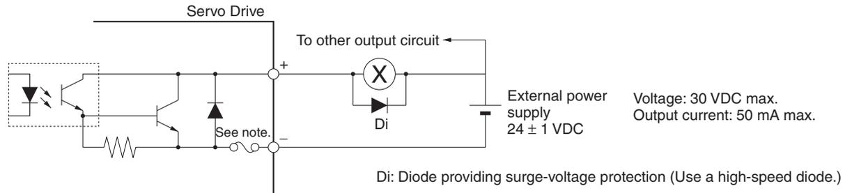
**Note** The circuit is equipped with an auto-resetting circuit breaker to protect the output. Even if an overcurrent trips the breaker, the breaker will reset automatically after a certain time elapses with no current.
