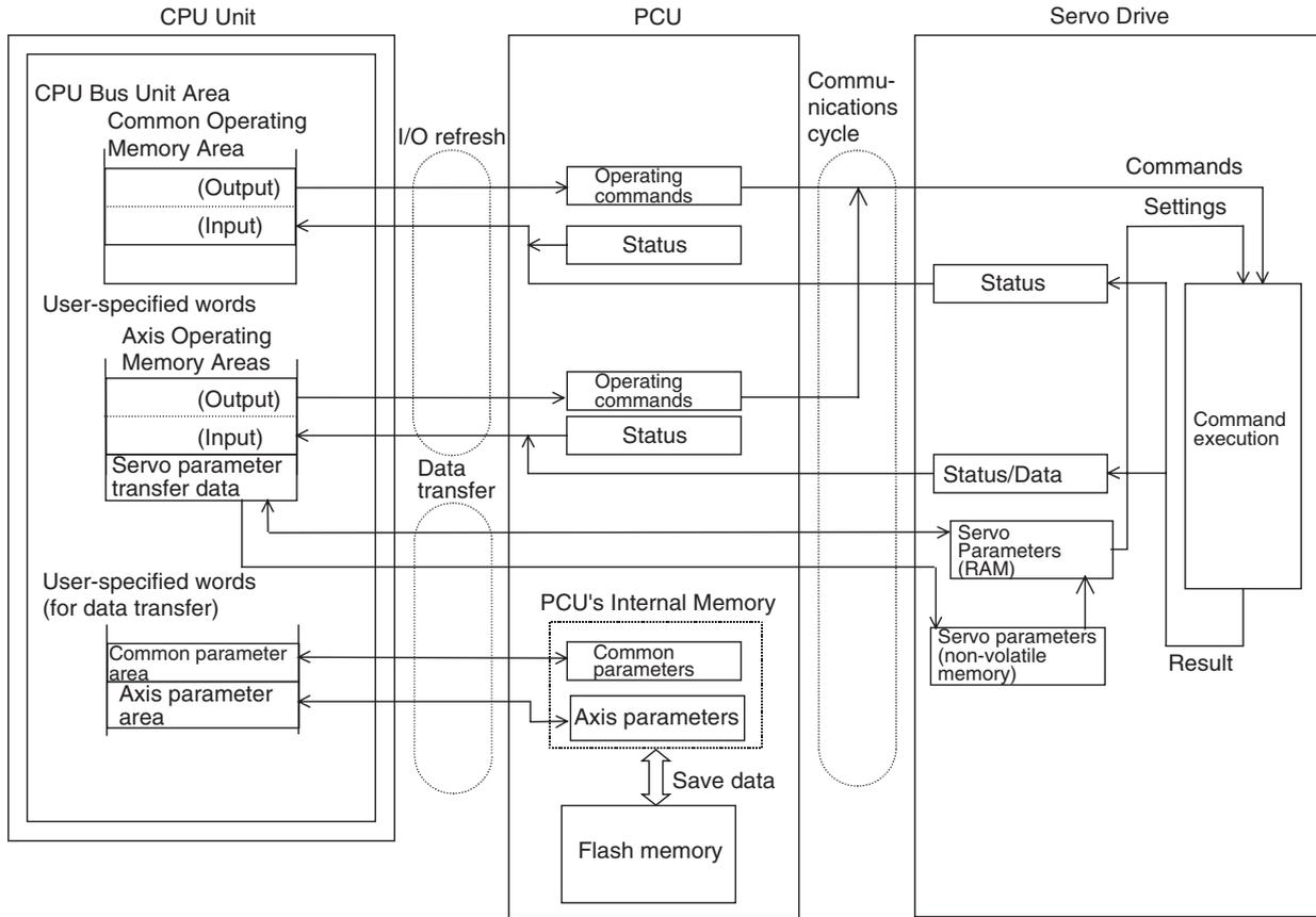
The data handled by the PCU can be classified into the following six types.
