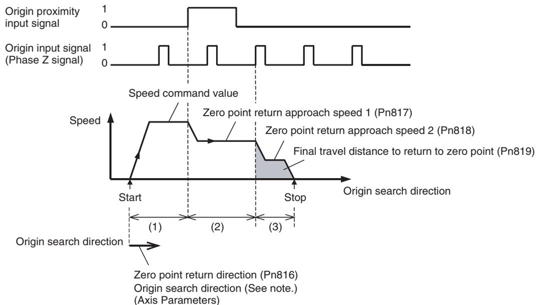
(1) The operation direction for origin search is determined by the setting in Servo Parameter *Zero Point Return Direction* (Pn816).
