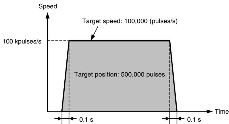
A Programming Console is used in this operation example without using a ladder program and with the PLC in PROGRAM mode to manually perform the settings and execute the start commands that are required to operate the Servomotor. The Programming Console is used to set the required data for direct operation and then turn ON the RELATIVE MOVEMENT Bit to operate the motor.
