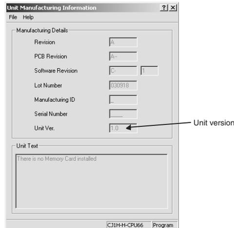
The unit version is displayed as 1.0 in the *Unit Version Number* field of the above example. Use the above display to confirm the unit version of the Unit connected online.
