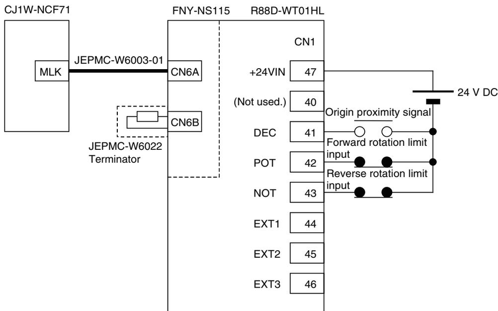
The Servo Drive's CN1 input signals depend on the input signal allocations, which are set in this operation example. Of these allocated input signals, the forward drive prohibit input (forward rotation limit input) and reverse drive prohibit input (reverse rotation limit input) are used as N.C. contacts. Therefore, connect them so that they are normally ON. The origin proximity signal and external latch inputs 1 to 3 are not used in this operation example and therefore do not need to be wired.
