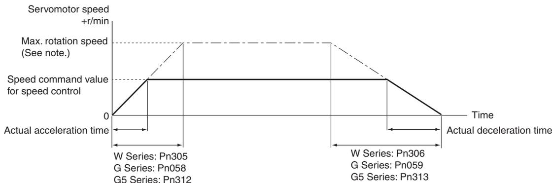
**Note** The maximum rotation speed depends on the Servomotor used. Refer to the maximum momentary rotation speed for the Servomotor used. The following values apply to W-series Servomotors.
