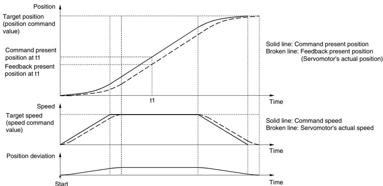
**Note** When executing speed control and torque control commands, there is no command present position because a positioning loop is not configured. A command present position calculated from the position deviation assumed from the current speed is output as monitor information.
