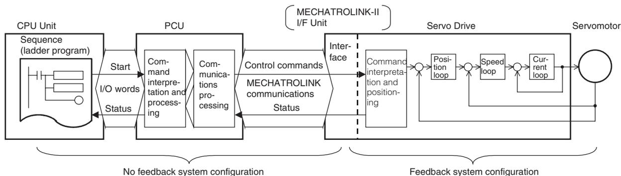
The control system configured using the PCU basically controls Servomotor operations using the semi-closed loop method. The semi-closed loop method detects the number of Servomotor rotations for the command value using the rotary encoder mounted to the Servomotor, and sends this feedback as the machine's travel distance. While calculating the deviation between the command value and actual number of Servomotor rotations, the machine is controlled so that the deviation is compensated to 0.
