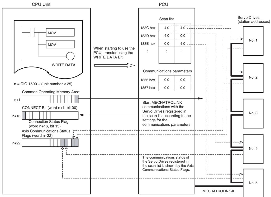
In the above example, Servo Drives are registered to axes 1, 2, 4, and 5 in the scan list (set to 40 hex). Therefore, MECHATROLINK communications start with the Servo Drives with station addresses No. 1, No. 2, No. 4, and No. 5 when CONNECT is executed.
