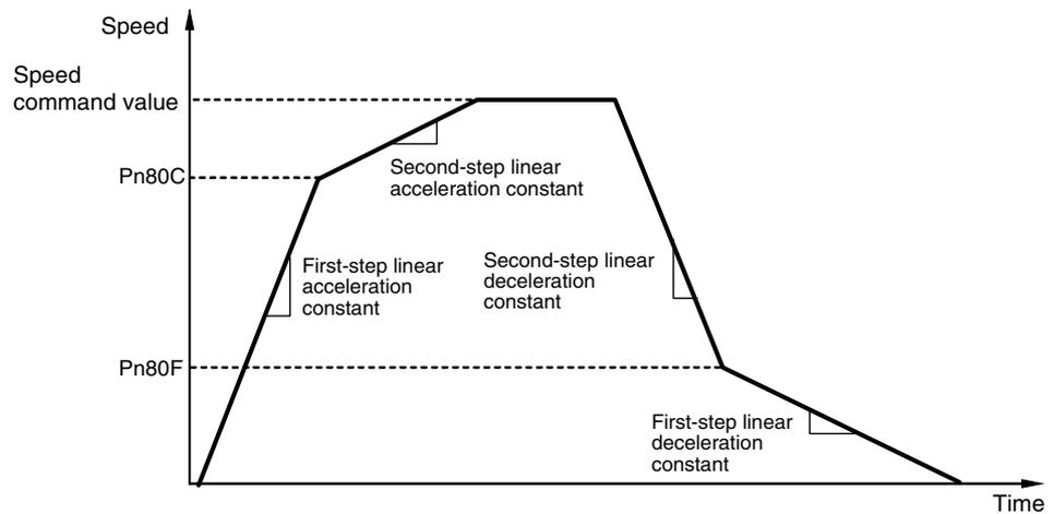
To operate an axis using only a first-step acceleration/deceleration curve with a W-series Servo Drive, only settings for the parameters Pn80B and Pn80E are required if the default settings (0) are used for the Servo Parameters *Acceleration Constant Switching Speed* and *Deceleration Constant Switching Speed* (Pn80C and Pn80F).
