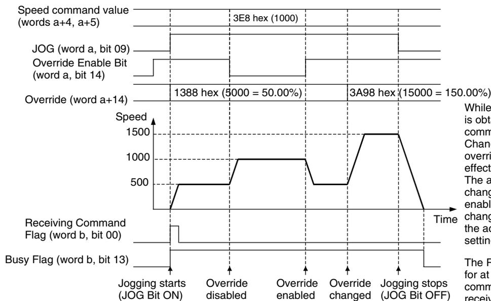
While override is enabled, the target speed is obtained by multiplying the speed command value by the override ratio. Changes to the override value while override is enabled are immediately effective in operations. The acceleration/deceleration used to change the speed when switching between enabling and disabling override or changing the override value depends on the acceleration/deceleration operation setting for the operation being performed.
