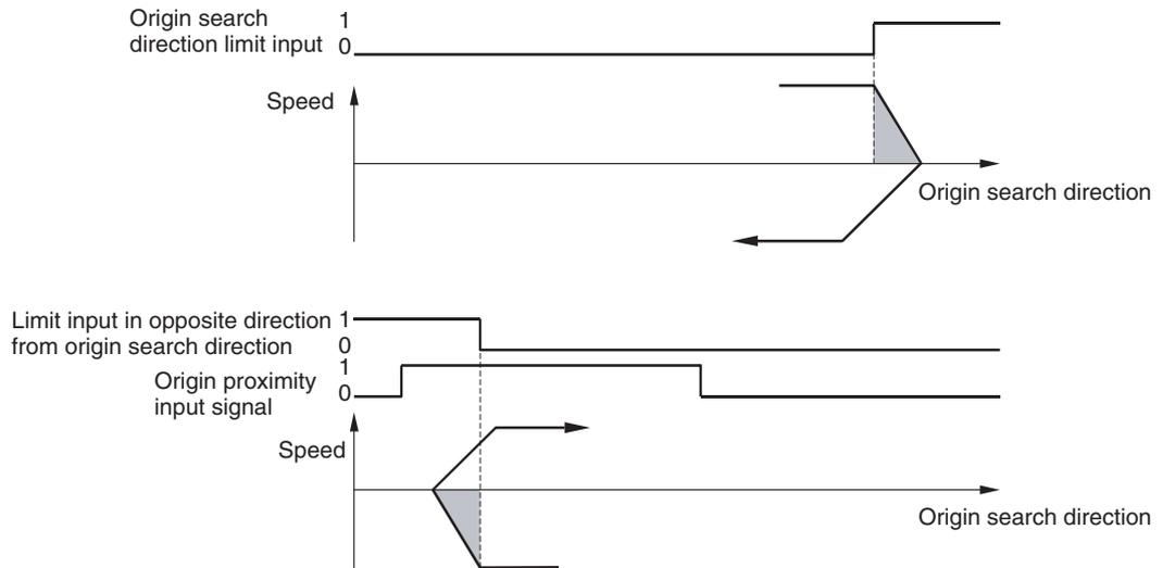
**Note** If the Servo Parameter (Pn505 for G5 Series, Pn066 for G Series and Pn001.1 for W Series) is set to stop operation with a free run when a limit input is input when using a G-series or a W-series Servo Drive, the momentum of the previous operation may cause the machine to run in the limit input direction.
