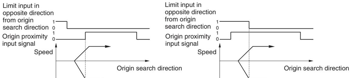
(2) The signal width of the origin input signal must be longer than the MECHATROLINK communications cycle when the Origin Proximity Input Signal parameter is set to 2 (Not use origin proximity input signal) during
