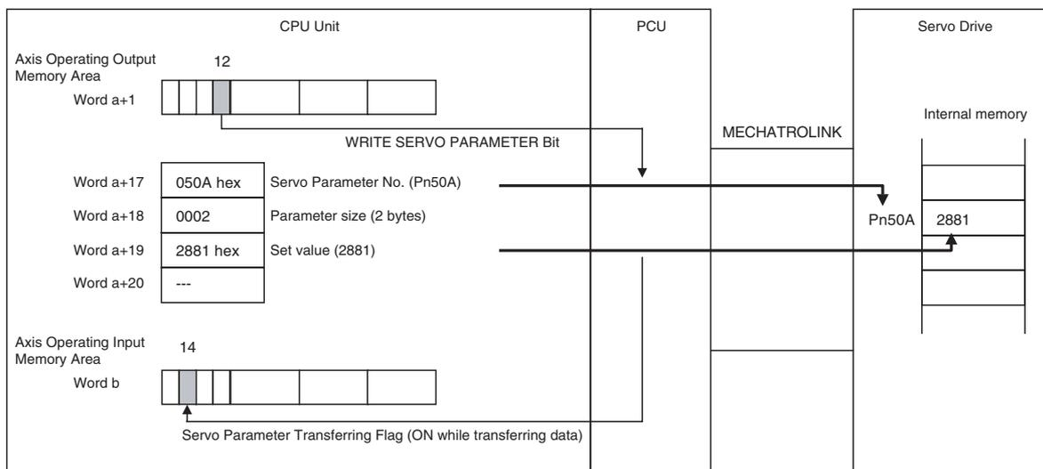
a = Beginning word of Axis Operating Output Areas specified in Common Parameters + (Axis No.-1) × 25
