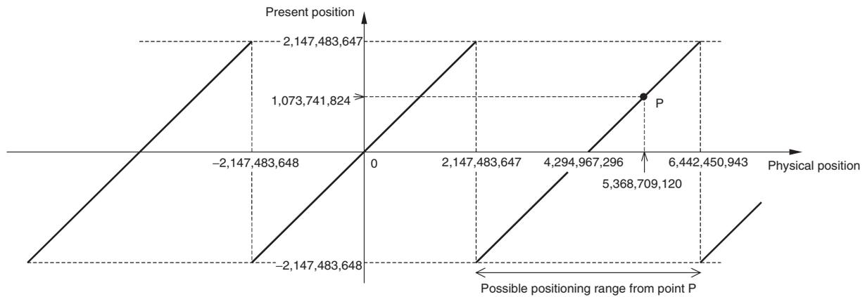
For example, if the physical position is 5,368,709,120 (command units), as indicated by point P in the above diagram, which exceeds 2,147,483,647 (command units), 1,073,741,824 will be given as the present position (command units).
