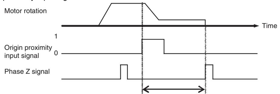
Provide a margin in the phase Z signal of at least two MECHATROLINK communications cycles plus 4 ms.
