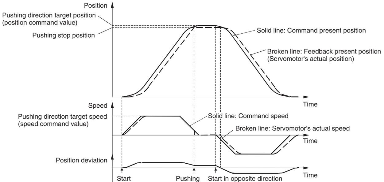
Alternatively, before performing the return operation, send a movement command to move the axis to the pushing stop position (feedback present position at pushing stop) and distribute the accumulated position deviation beforehand, as shown in the following diagram.
