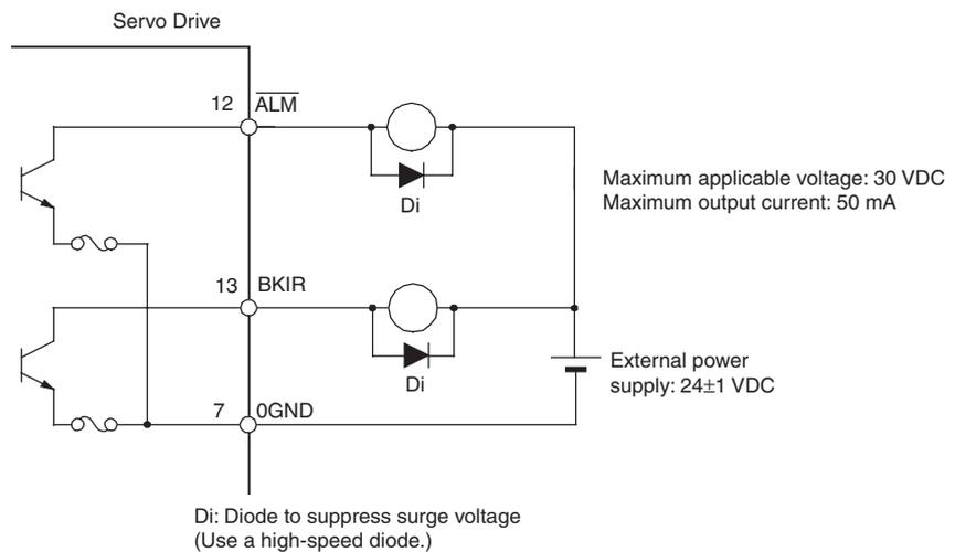
**Note** The circuit is equipped with an auto-resetting circuit breaker to protect the output. Even if an overcurrent trips the breaker, the breaker will reset automatically after a certain time elapses with no current.
