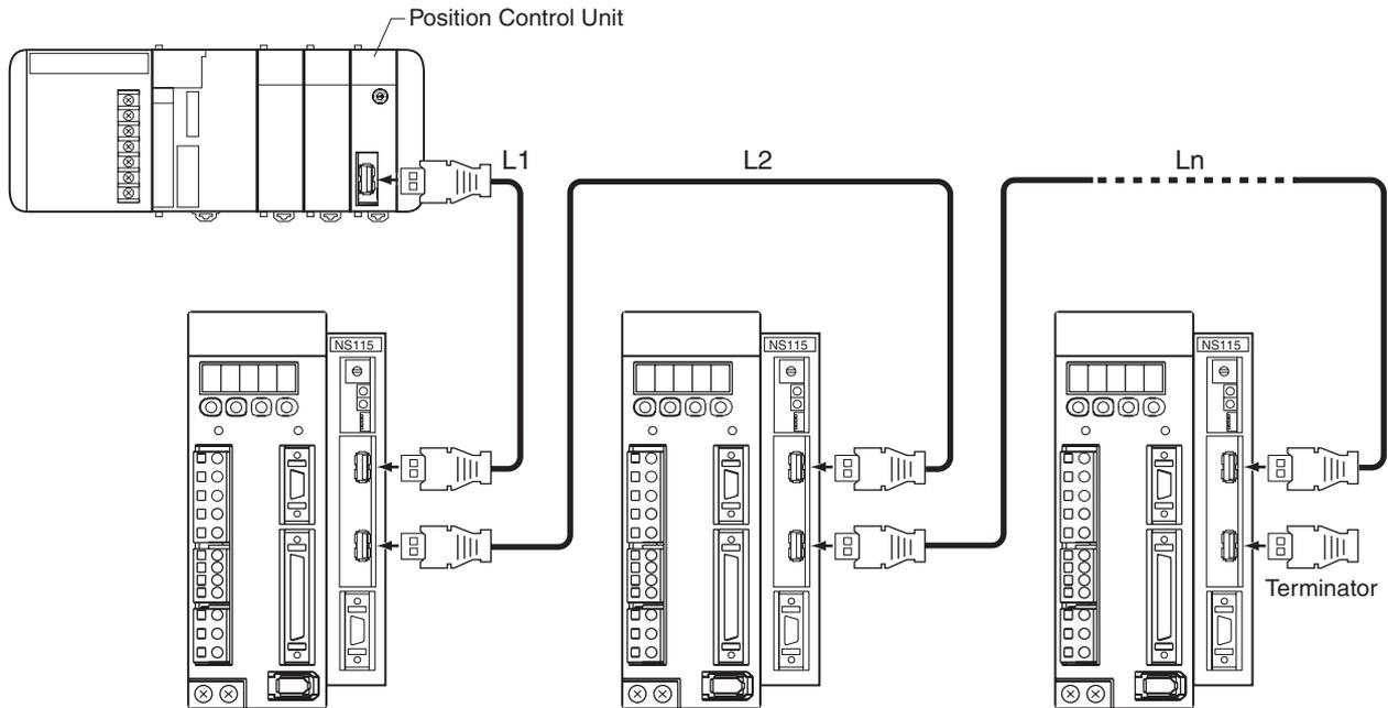
**Note** When not using Repeaters, the maximum total length of the Connection Cable ( $L1 + L2 + \dots + Ln$ ) is 50 m when using fewer than 16 axes or 30 m when using 16 axes.
