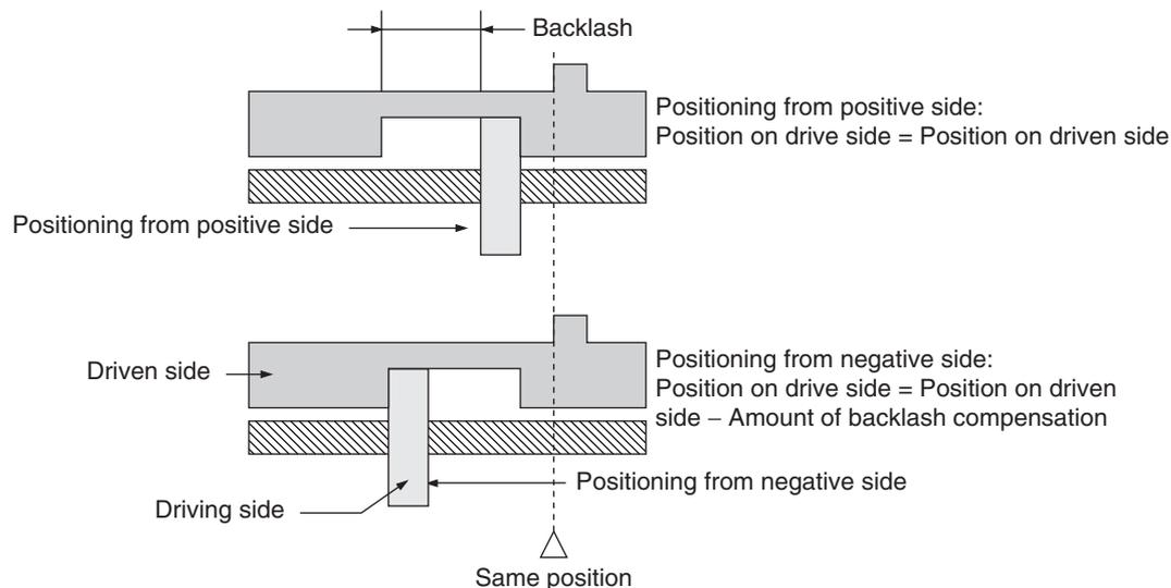
In the above diagram, after positioning from the positive side, backlash is compensated for up to the amount of the output of pulses set for the backlash compensation either when positioning in the negative direction or when the positioning direction is reversed.
