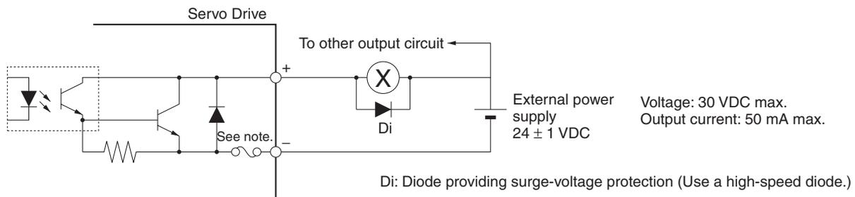
**Note** The circuit is equipped with an auto-resetting circuit breaker to protect the output. Even if an overcurrent trips the breaker, the breaker will reset automatically after a certain time elapses with no current. (Ver. 37 and later Servo Drives are equipped with the auto-resetting circuit breakers.)
