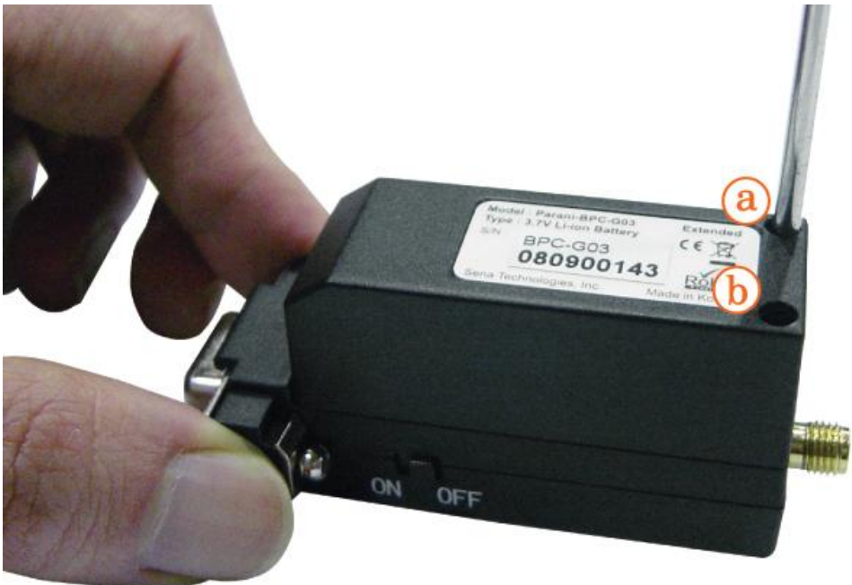
Figure 2-7 Fasten the battery pack
