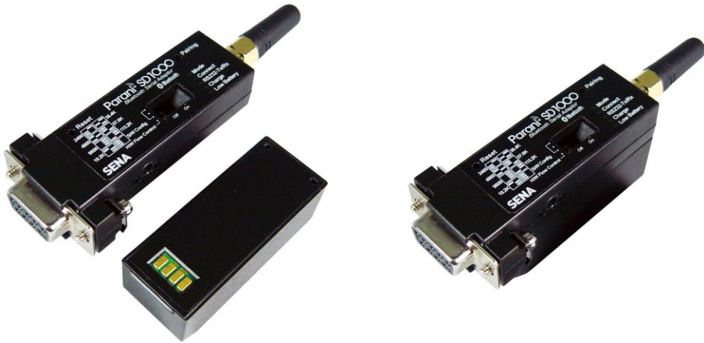
Figure 2-4 Attaching Battery Pack to Parani-SD1000
