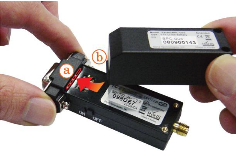
Figure 2-6 Attach the battery pack
