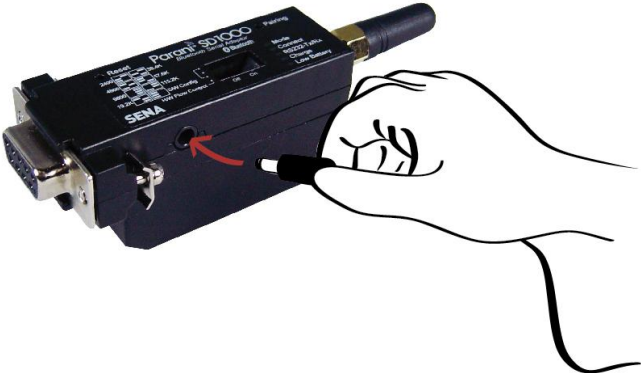
Figure 2-2 Connecting Power to Parani-SD1000
