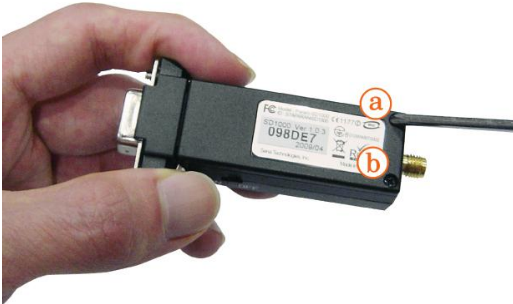
Figure 2-5 Remove Parani-SD1000 bottom cover
