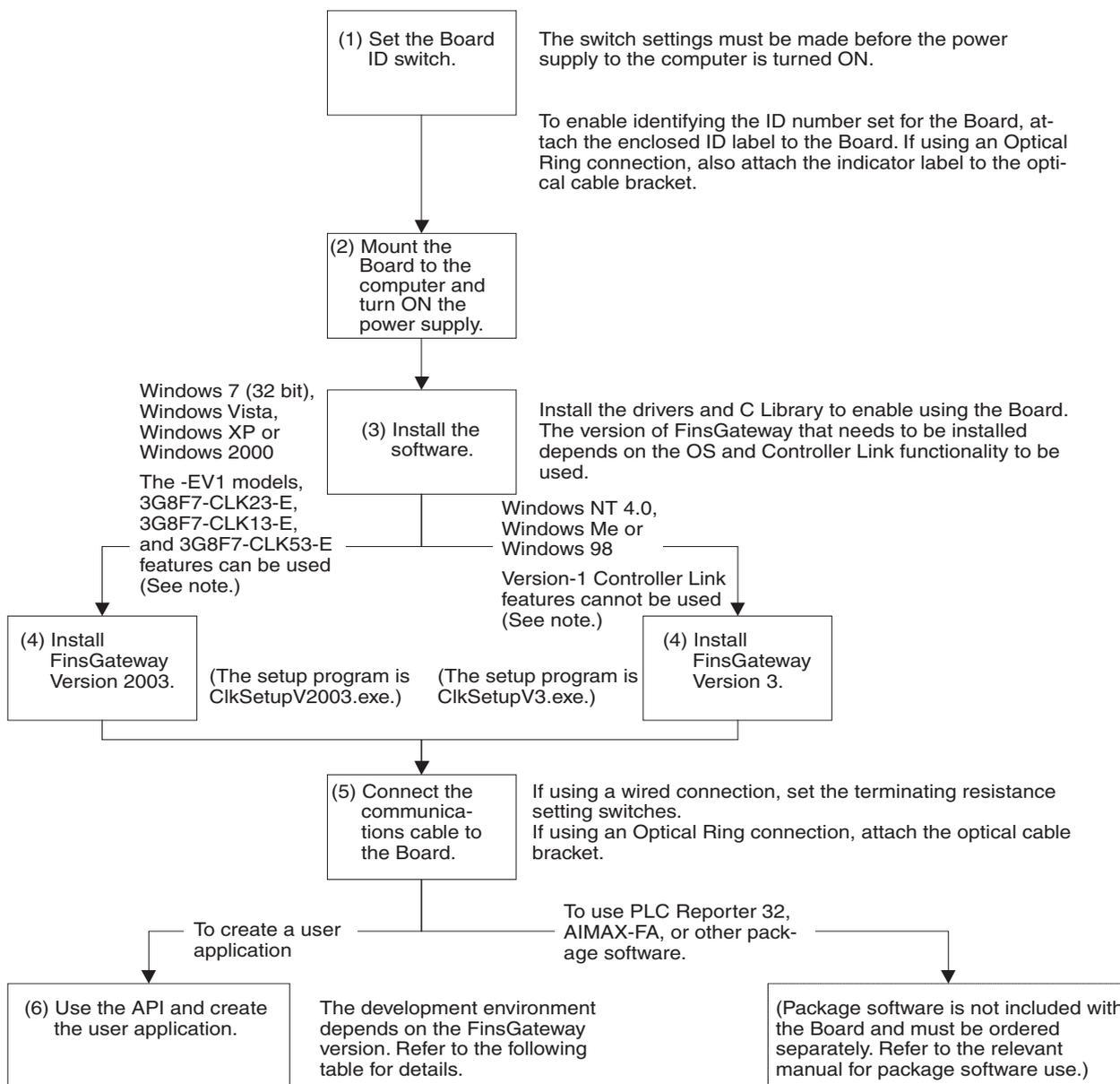
**Note** The new version-1 Controller Link functionality is as follows: Automatic 1:N data link allocations, support for 62 wired nodes, and data link table changes with active data links. Maximum number of data link send words per node: 4,000
