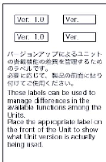
These labels can be affixed to the front of earlier Controllers to differentiate between Controllers with different unit versions.
