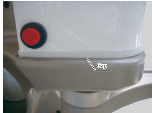
Gap at bottom of cover
