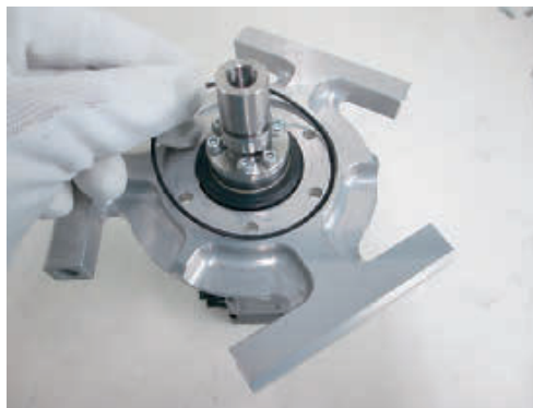
▶ Step 7 Seal removal
