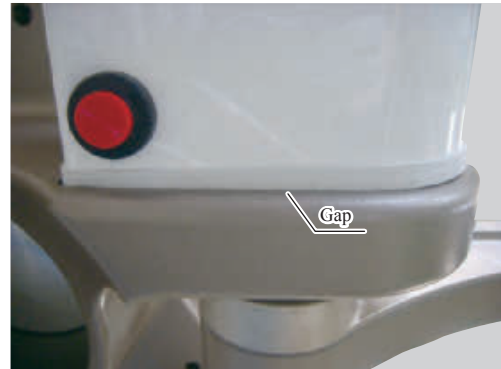
Gap at bottom of cover
