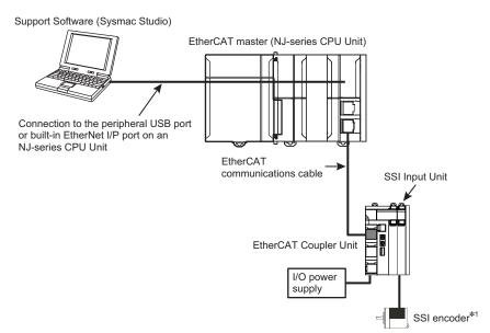
\*1. The SSI encoder is supplied with 24-VDC power from the SSI Input Unit.
