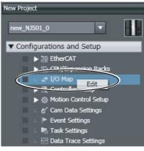
2 Select the I/O port on the I/O Map Tab Page and enter the variable name in the Variable Column.
