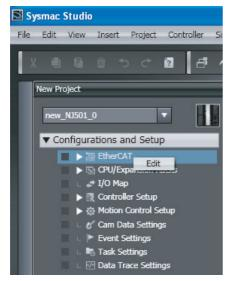
**3** Right-click the EtherCAT master that is displayed in the Edit Pane and select *Write Slave Node Address*.
