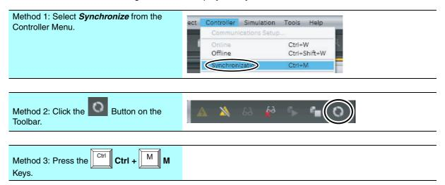
Comparison of the data on the computer and the data in the physical Controller is started.
