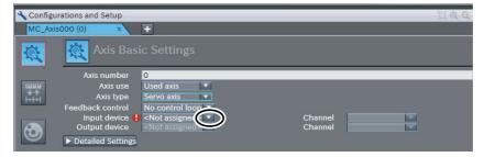
This will assign node 1 and device R88D-KN01L-ECT as the input device for axis 0.
