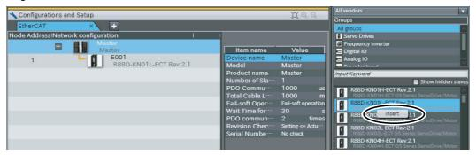
The Servo Drive is added under *E001* with a node address of 2.
