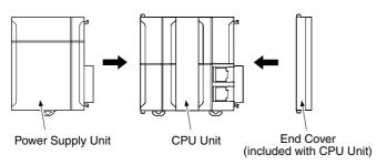
After joining the connectors between the Units, use the sliders at the top and bottom of each Unit to lock the Units together. Lock the sliders firmly into place.
