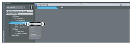
The local variable table and Ladder Editor are displayed in the Edit Pane. From here, you can register local variables and create a ladder diagram.
