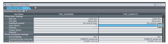
Now, node 2 with device R88D-KN01L-ECT can be used as an axis in the EtherCAT network configuration.
