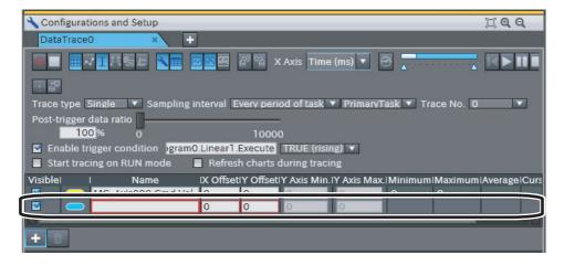
4 Enter MC Axis001.Cmd.Vel for the name of the variable to trace on the new line.
