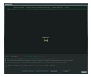
The following dialog box is displayed when the transfer is completed. Click the  $\bf No$  Button. Do not change to RUN mode at this time (i.e., remain in PROGRAM mode).
