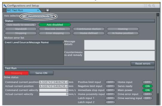
Check to see if the signals turn ON and OFF properly on the monitor screen by turning ON and OFF the sensor connected to each control input signal.
