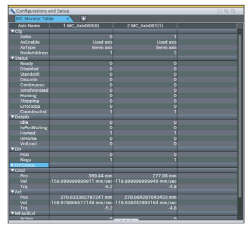
Use the MC Monitor Table to confirm that the axis 0 and axis 1 are moving.a and b in the following figure show the information you need to check.a: Check that the value of *Pos* under *Cmd* is either increasing or decreasing.
