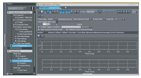
Select the Enable trigger condition Check Box on the DataTrace0 Tab Page and enter the variable to use as the trigger condition. For this example, use *Program0.Move1.Execute*.
