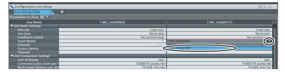
This will assign node 2 and device R88D-KN01L-ECT as the input device for axis 1.
