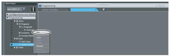
The local variable table and Ladder Editor are displayed in the Edit Pane. From here, you can register local variables and create a ladder diagram.
