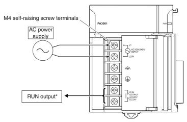
\* The RUN output is ON when the CPU Unit is in RUN mode. It is OFF when the CPU Unit is in PROGRAM mode or when a major fault level Controller error occurs.
