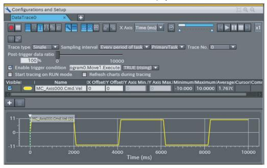
Make sure that the trace results show the same waveform as shown in 3-1 Single-axis Servo System Operation.
