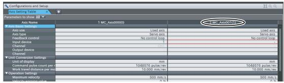
In this state, the input device for axis 1 still needs to be assigned to a Servo Drive.
