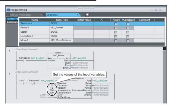
Insert the second MC MoveRelative (Relative Positioning) instruction. Enter Move2 as the instance name, enter the axis variable of axis 0 (MC\_Axis000) for the in-out variable, and enter the values in the following table for the input variables.
