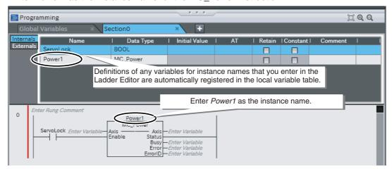
Enter the in-out variable for the Power1 instance.
