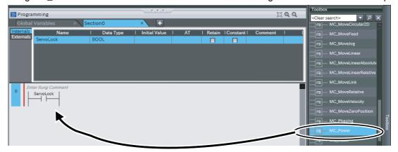
An MC\_Power instruction is inserted to the right of the ServoLock input.
