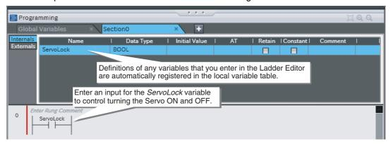
**2** Drag MC\_Power from the Motion Area of the Toolbox to the right side of the ServoLock input.
