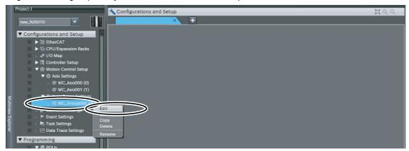
The axes group settings are displayed on the Axes Group Basic Settings Display in the Edit Pane.
