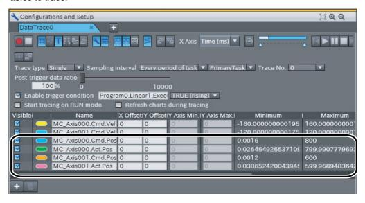
**5** Select the *Enable trigger condition* Check Box on the DataTrace0 Tab Page and enter the *Program0.Linear1.Execute* variable to use as the trigger condition.
