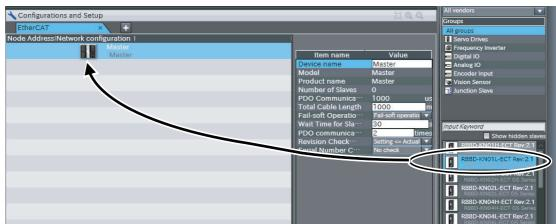
**2** Drag the R88D-KN01L-ECT from the Toolbox to the master on the EtherCAT Tab Page.
