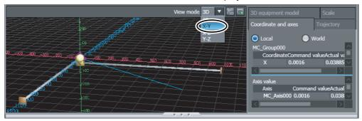
The results of the data trace are displayed in Cartesian coordinates with axis 0 as the X axis and axis 1 as the Y axis.
