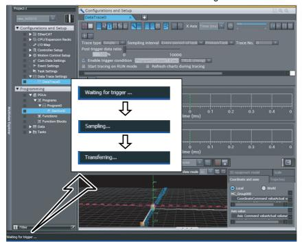
The results of the data trace are displayed on the 3D Motion Trace Display.
