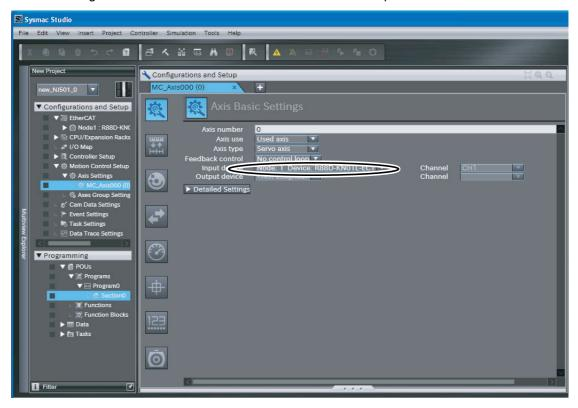
Now, node 1 with device R88D-KN01L-ECT can be used as an axis in the EtherCAT network configuration.
