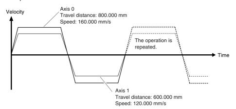
The axis created in Section 3 Setting Up a Single-axis Servo System is axis 0. The axis added in this section is axis 1.
