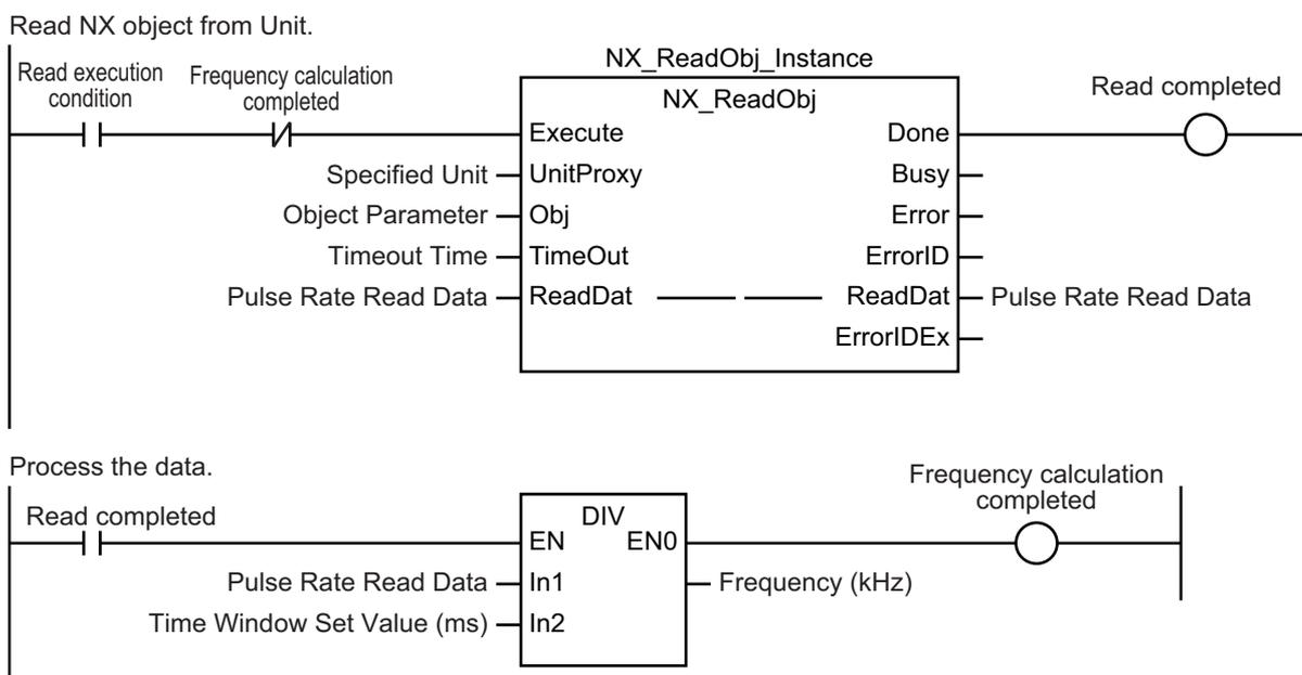
In this example, the time window set value (unit: ms) in the Incremental Encoder Input Unit is used as it is in the frequency calculation. The unit of the calculated frequency is therefore kHz.
