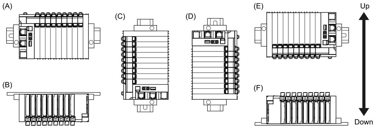
However, there are restrictions on the installation orientation and restrictions to the specifications that can result from the Communications Coupler Units and NX Units that are used.
