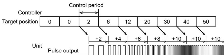
The frequency is calculated based on the travel distance for the control period and the pulses are output.
