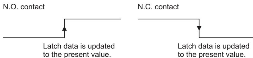
You can assign up to two external inputs as latch inputs, each with an I/O data input area allocation.
