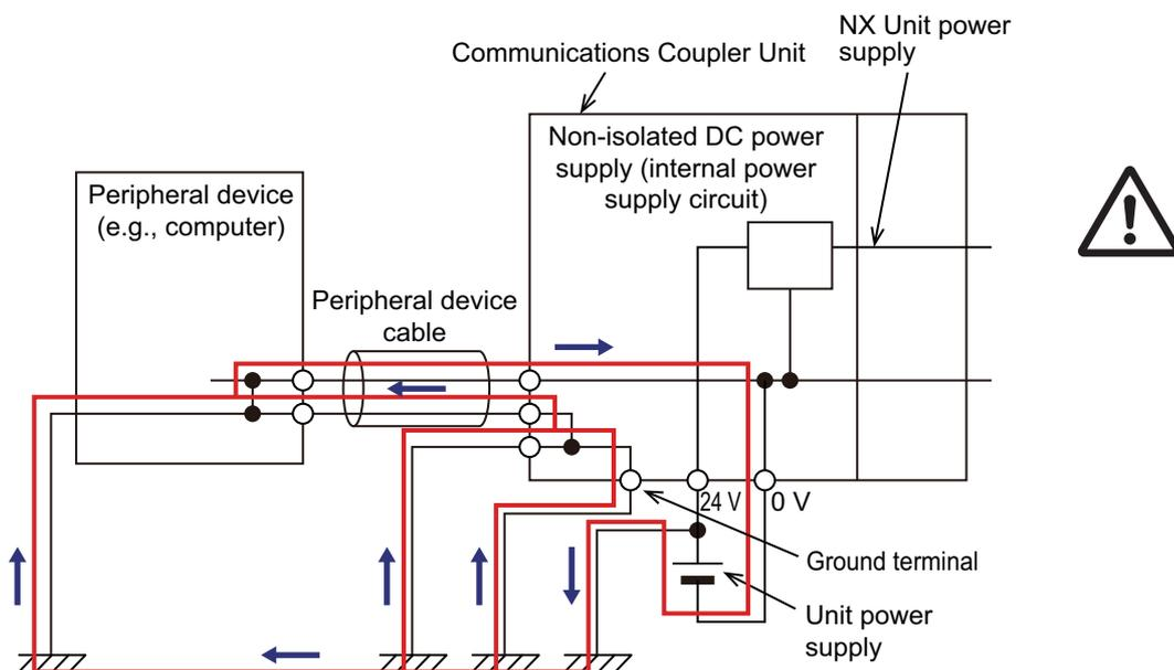
Be sure that all terminal screws and cable connector screws are tightened to the torque specified in the relevant manuals. The loose screws may result in fire or malfunction.
