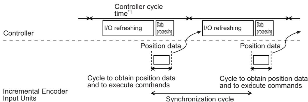
\*1. For an NX-series CPU Unit, the task period of the primary periodic task or priority-5 periodic task is applicable. For an NJ-series CPU Unit, only the task period of the primary periodic task is applicable.
