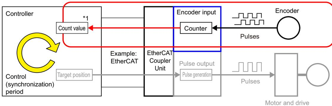
\*1. The count value of the encoder (pulses) is sent to the Controller every control period.
