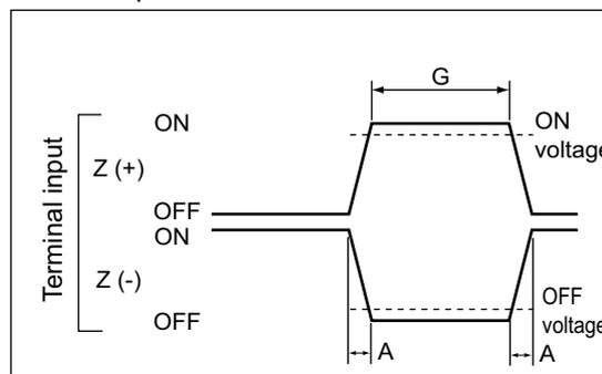
Relationship between Phase A and Phase B on Phase Differential Pulse Inputs
