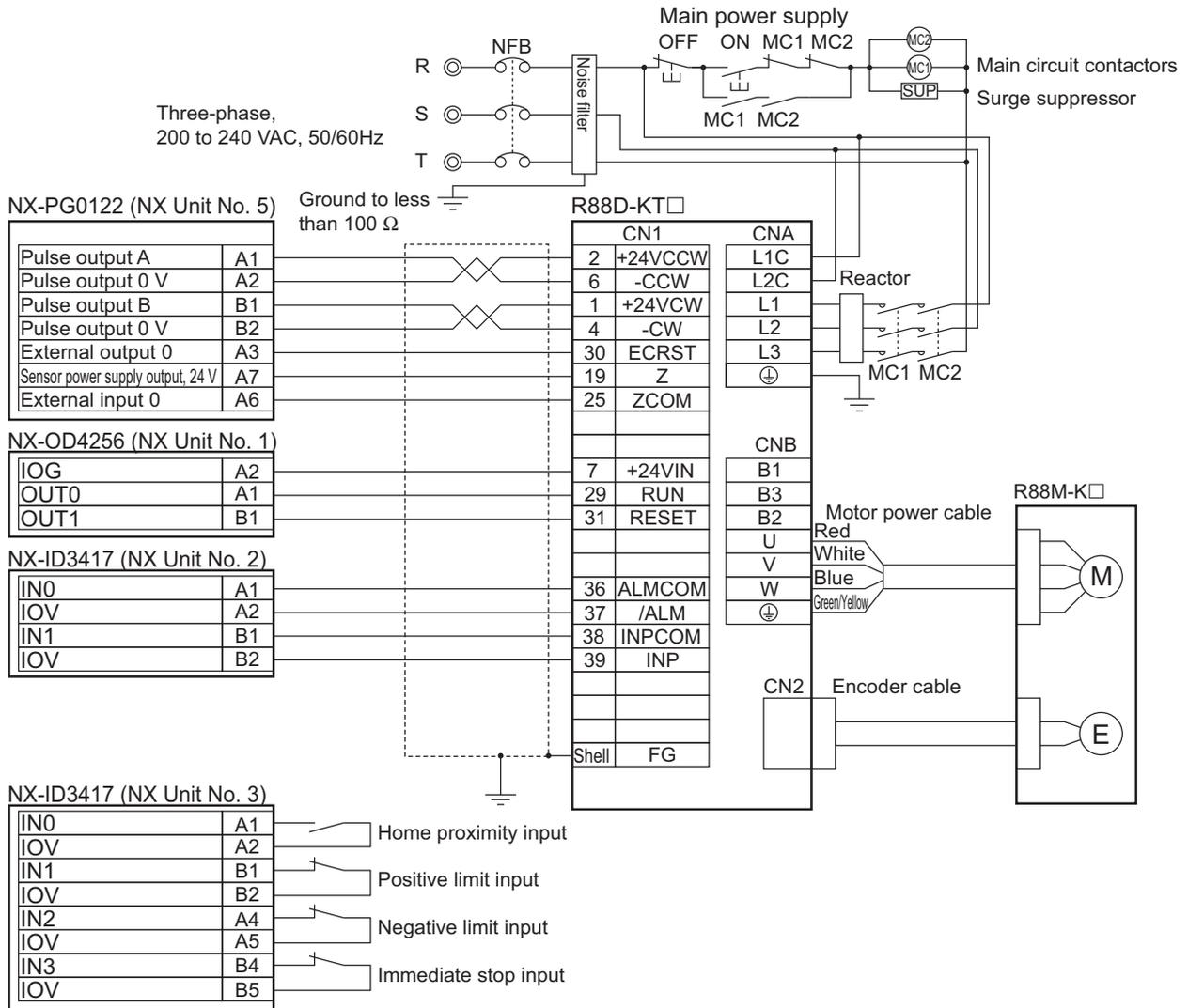
The external output 0 (O0) from the NX-PG0122 Pulse Output Unit is a PNP output. In this example, it is used as an error counter reset output.
