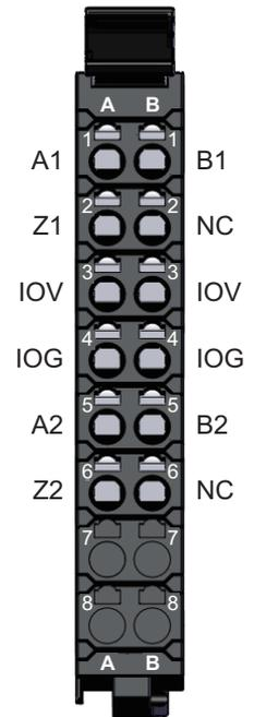
Note The encoder power supply output (24 V and 0 V) is provided power from the I/O power supply connected to the Communications Coupler Unit or an Additional I/O Power Supply Unit.
