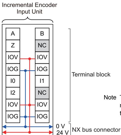
Note The I/O power is supplied from the I/O power supply connected to the I/O power supply terminals on the Communications Coupler Unit or an Additional I/O Power Supply Unit.
