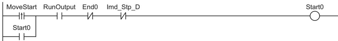
When the relative positioning instruction is completed and the *InPosition* input changes to TRUE, the positioning completion condition, *End0*,
