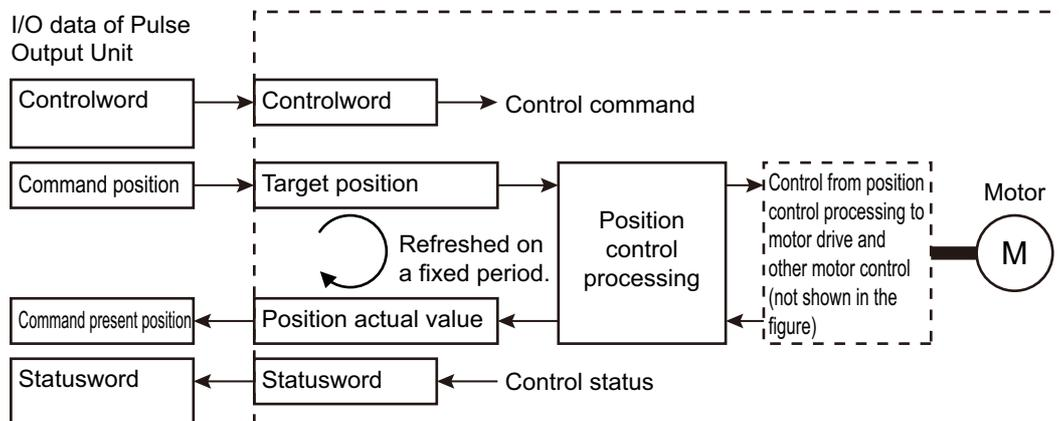
In Cyclic Synchronous Position Control Mode, motor position control is performed by sending the motor target position on a fixed synchronization cycle. The result of that operation is monitored as the position actual value.
