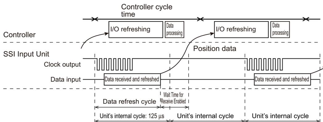
For this method, the SSI Input Unit sends a clock signal to the encoder that is timed to the internal cycle of the Unit and receives data from the encoder.
