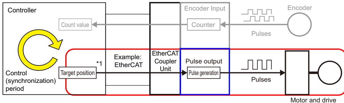
\*1. Pulse output is performed based on the synchronization commands (target positions) received from the Controller each control period.
