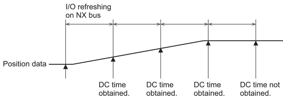
The obtained position data and DC time are input to the Controller.
