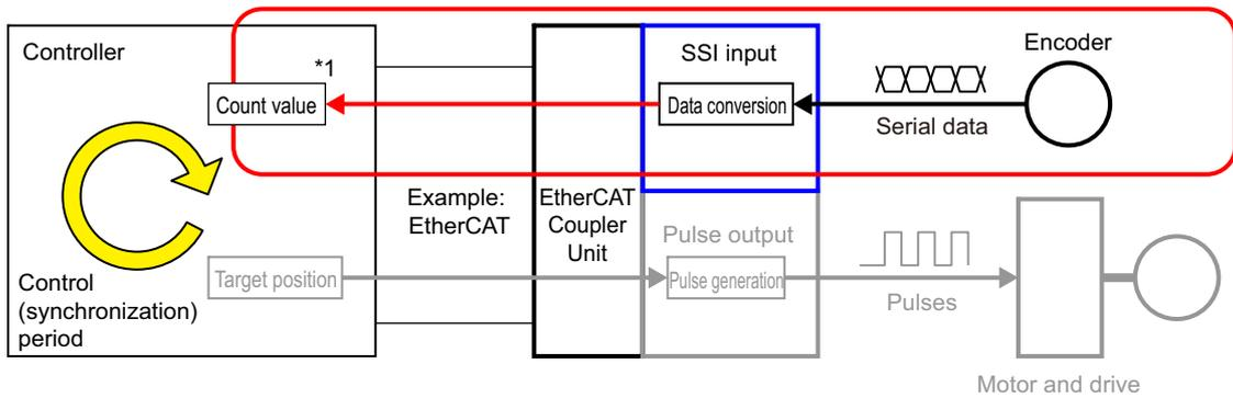
\*1. The count value of the encoder (serial data) is sent to the Controller every control period.
