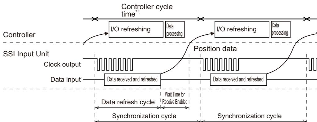
\*1. For an NX-series CPU Unit, the task period of the primary periodic task or priority-5 periodic task is applicable. For an NJ-series CPU Unit, only the task period of the primary periodic task is applicable.
