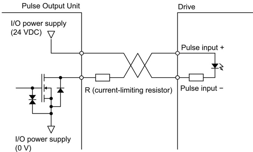
● **OMRON G5-series Servomotor/Servo Drive Wiring Example**
