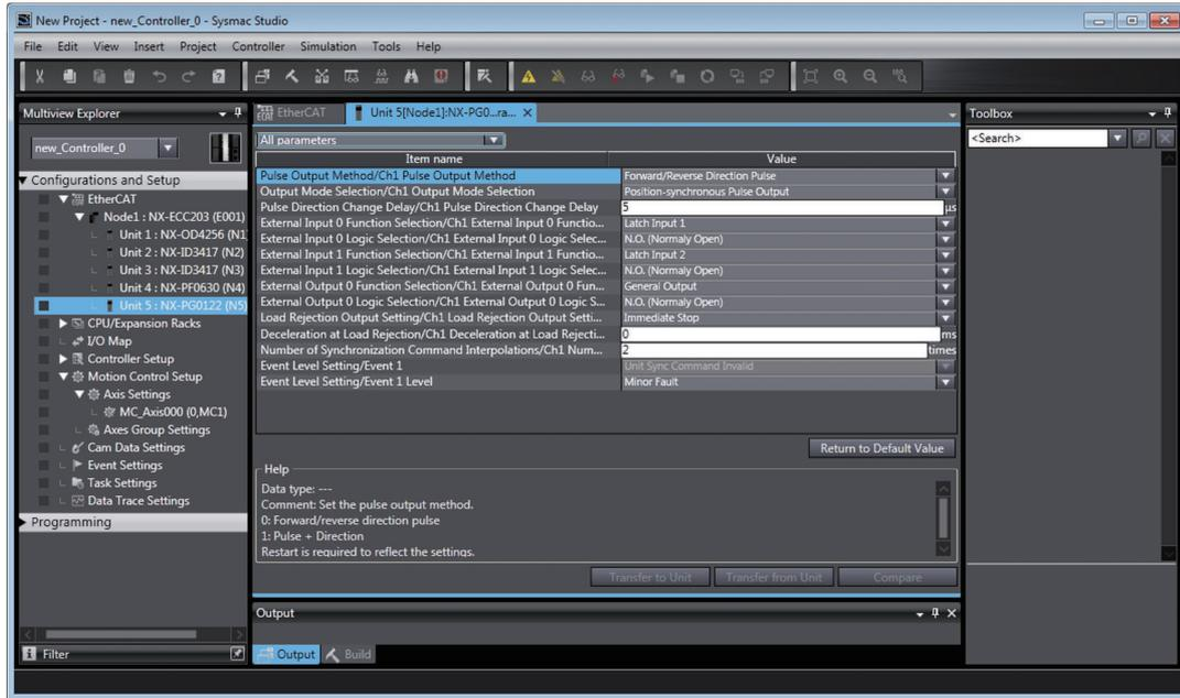
**2** Set the External Input 0 Function Selection and External Input 1 Function Selection parameters.
