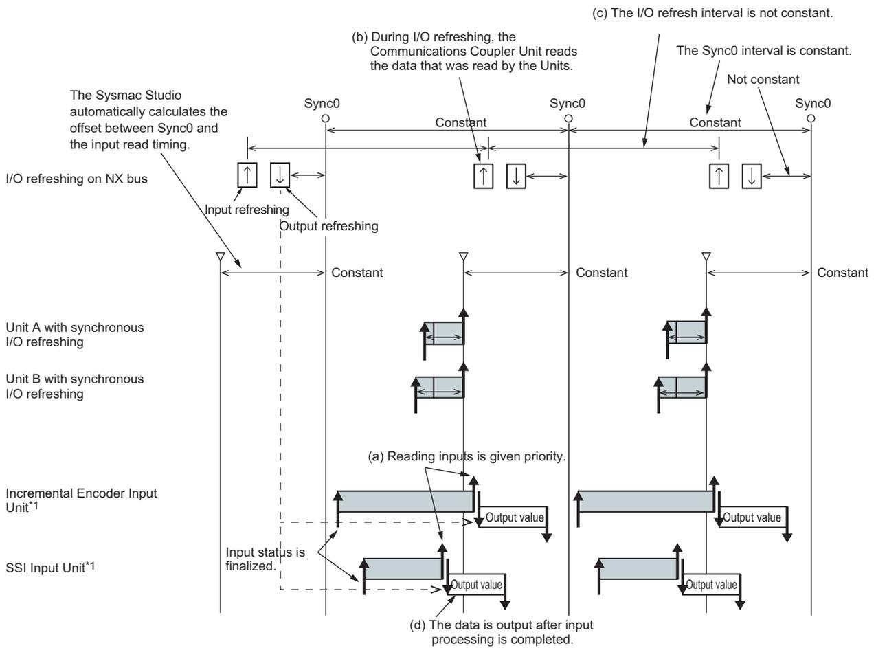
\*1. The timing of I/O is given as an example. The actual timing will vary.
