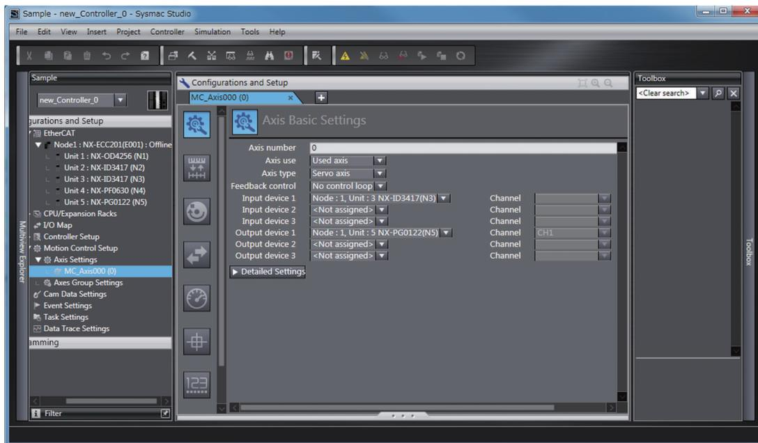
The following default I/O entry mappings are set as the process data assignments for the Pulse Output Unit and the process data is automatically assigned to the appropriate axis functions.
