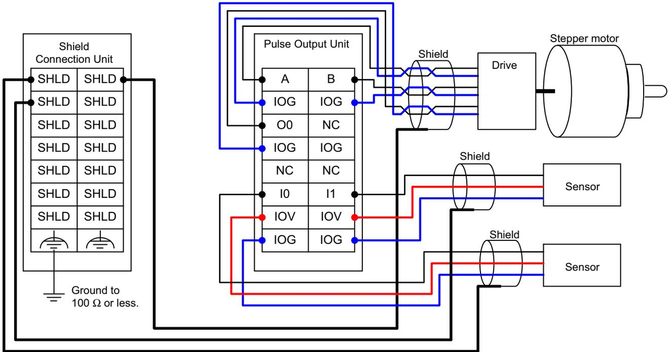
Note The pulse output from an NX-PG0122 Pulse Output Unit is a 24-VDC PNP output. Refer to *8-6 Terminal Block Arrangement* on page 8-14 for information on wiring drives.
