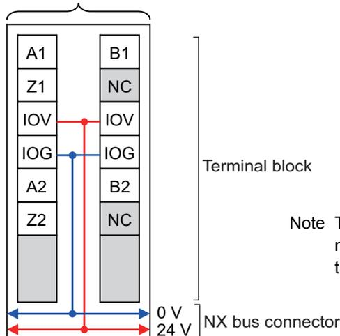
Note The I/O power is supplied from the I/O power supply connected to the I/O power supply terminals on the Communications Coupler Unit or an Additional I/O Power Supply Unit.
