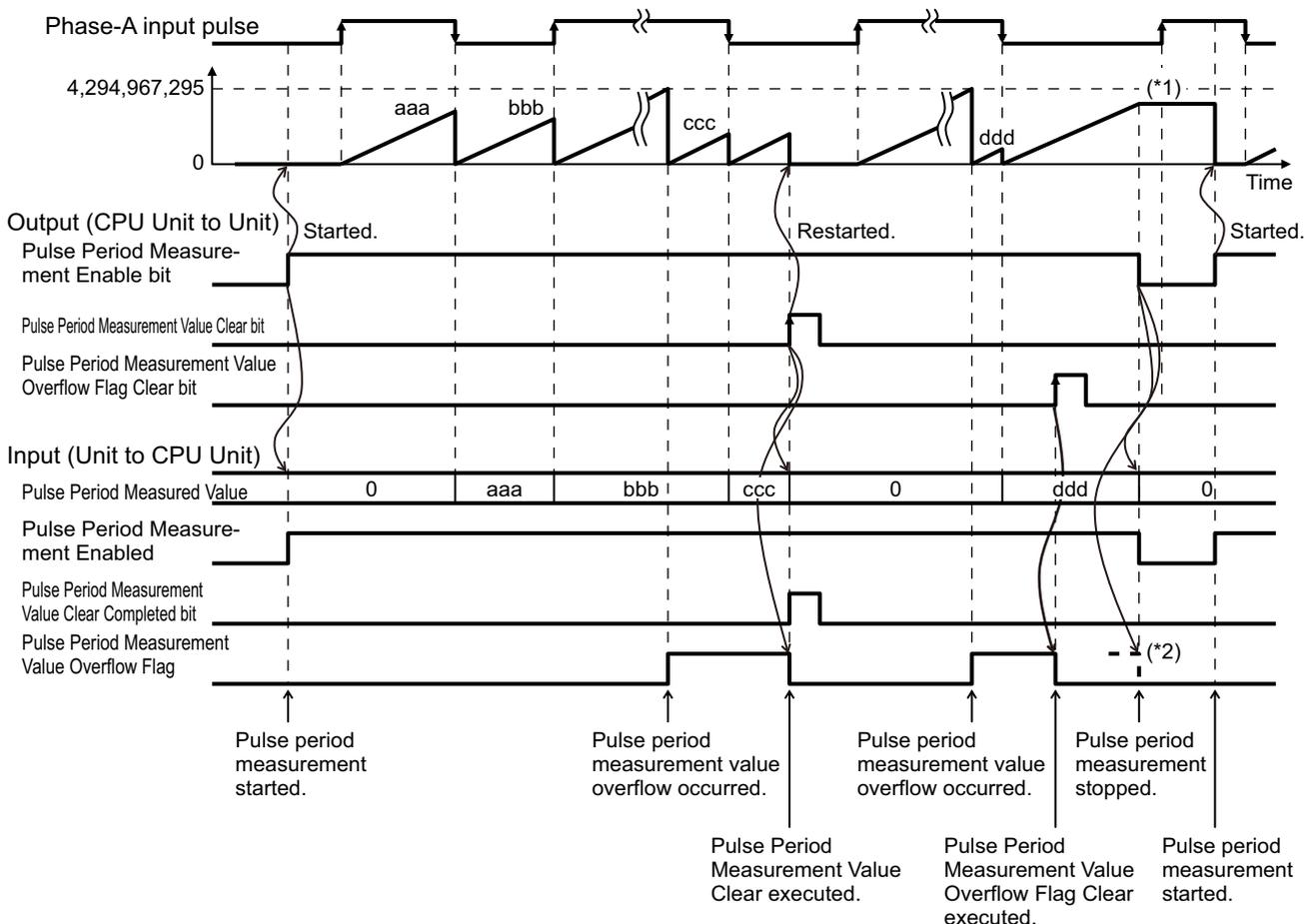
\*1. The pulse period measurement counter retains the most recent value while the function is disabled.
