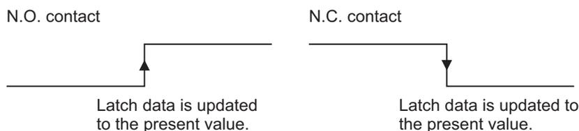
You can assign up to two external inputs as latch inputs, each with an I/O data input area allocation.
