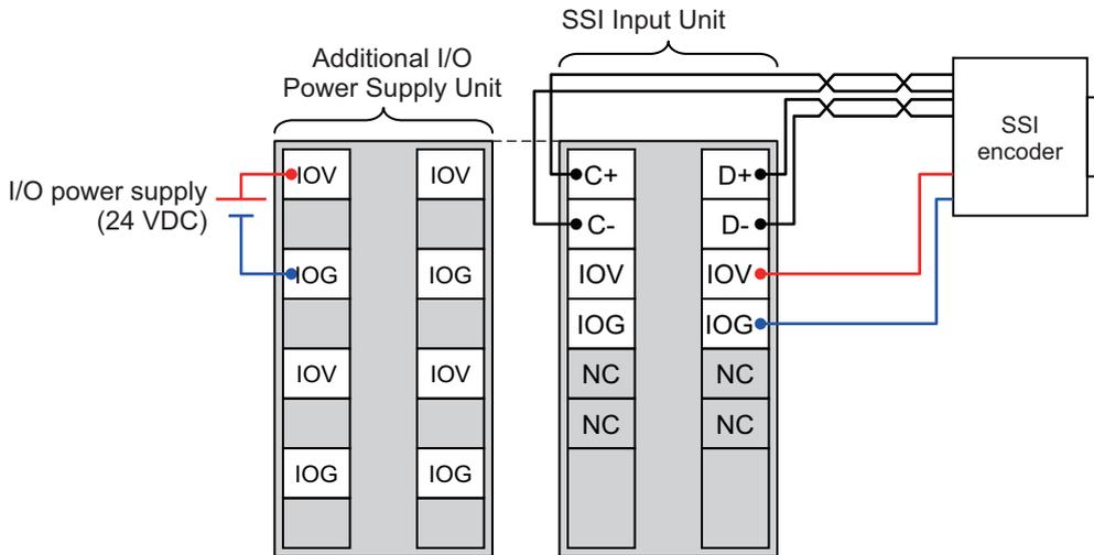
Note To supply power to connected external devices, connect an 24-VDC I/O power supply to the Communications Coupler Unit or an Additional I/O Power Supply Unit to supply power to the SSI Input Unit.
