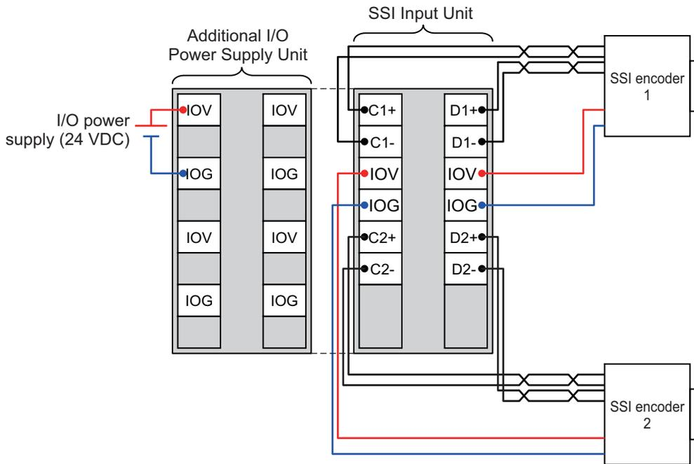
Note To supply power to connected external devices, connect an 24-VDC I/O power supply to the Communications Coupler Unit or an Additional I/O Power Supply Unit to supply power to the SSI Input Unit.
