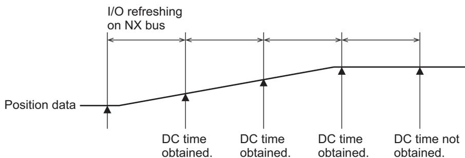
The obtained position data and DC time are input to the Controller.
