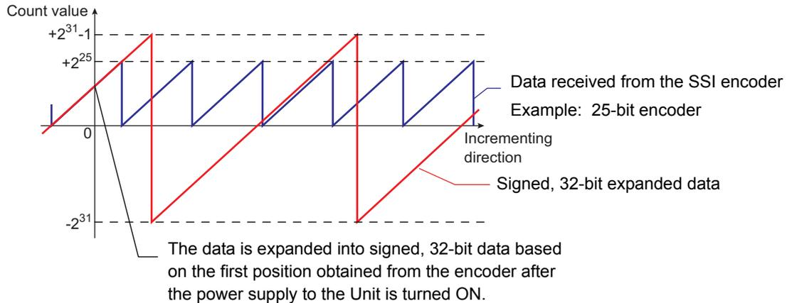
If you use present value conversion with an SSI encoder that supports a resolution other than 32 bits, the reference point (home position) changes from the signed, 32-bit data after one rotation of absolute value data from the encoder.
