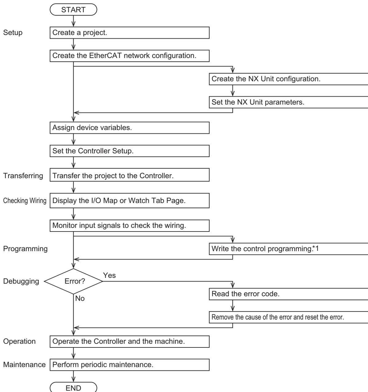
\*1. If the MC Function Module is not used, all control tasks must be performed in the user program, including position management.
