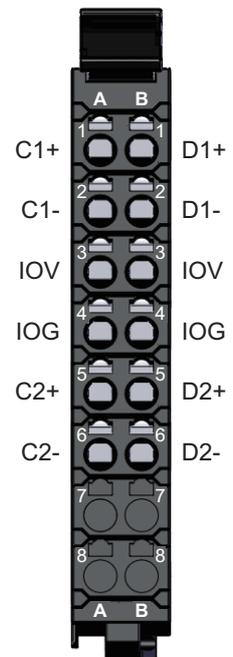
Note The SSI power supply output (24 V and 0 V) is provided power from the I/O power supply connected to the Communications Coupler Unit or an Additional I/O Power Supply Unit.
