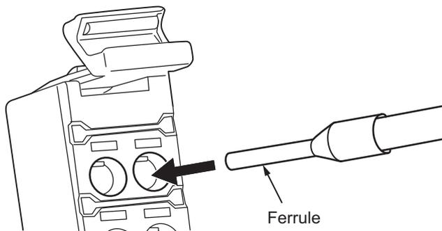
After you make a connection, make sure that the ferrule is securely connected to the terminal block.
