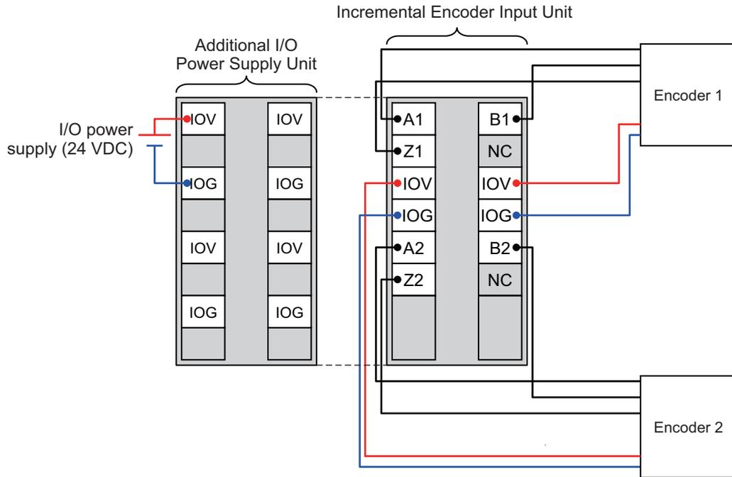
Note 1. The encoder inputs on Units with voltage inputs are PNP connections.
