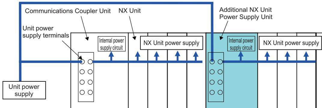
The power supply capacity of the Communications Coupler Unit is not sufficient for the following Units.
