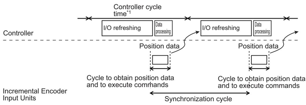
\*1. For an NX-series CPU Unit, the task period of the primary periodic task or priority-5 periodic task is applicable. For an NJ-series CPU Unit, only the task period of the primary periodic task is applicable.
