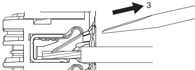
After you make a connection, make sure that the twisted wire or the solid wire is securely connected to the terminal block.
