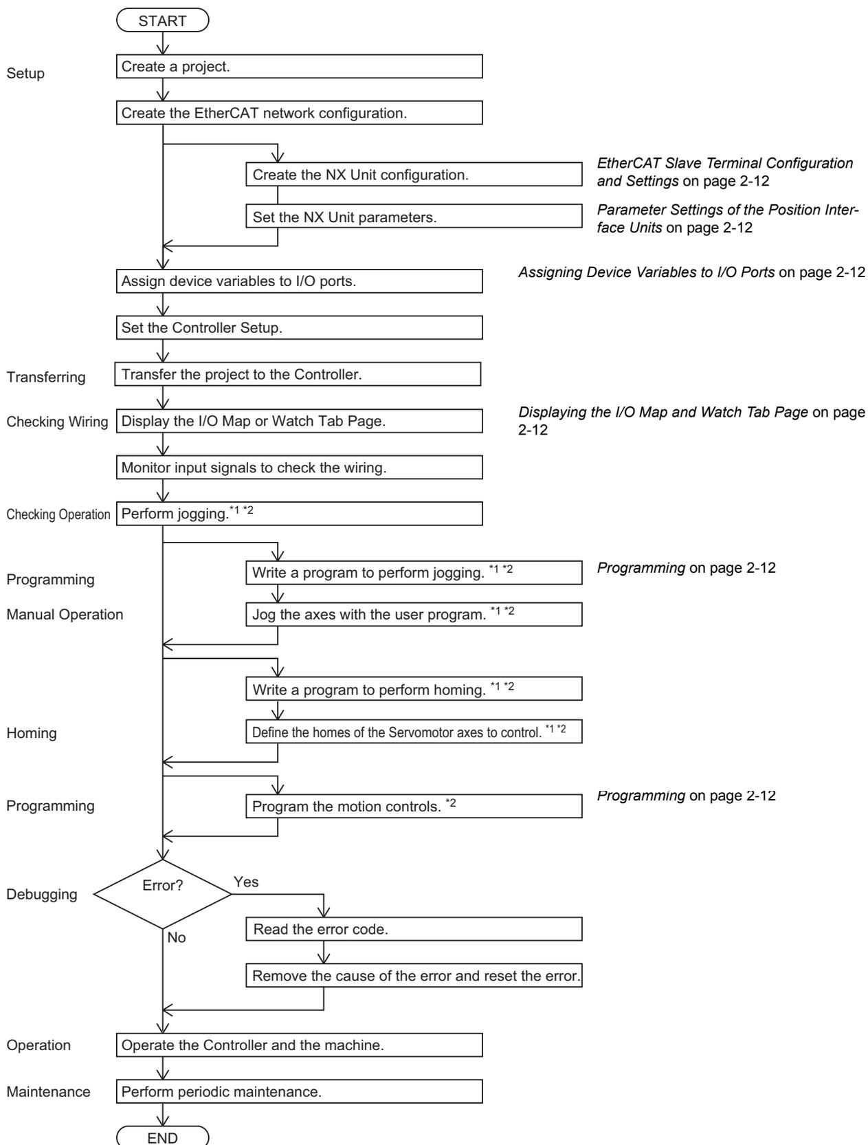
\*1. These steps are required if a Pulse Output Unit is used to control the motor drive.
