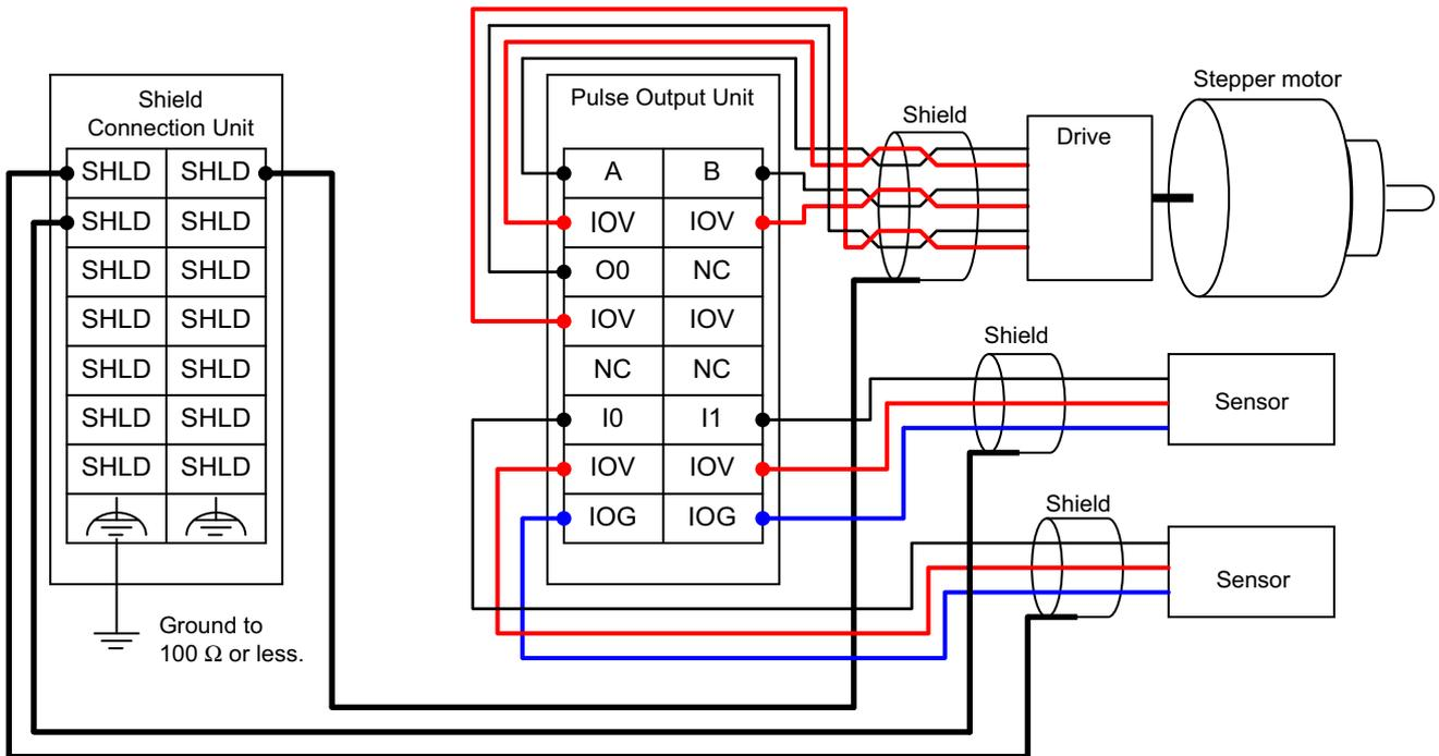
Note The pulse output from an NX-PG0112 Pulse Output Unit is a 24-VDC NPN output. Refer to 8-6 *Terminal Block Arrangement* on page 8-14 for information on wiring drives.
