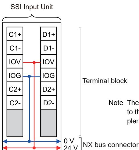
Note The I/O power is supplied from the I/O power supply connected to the I/O power supply terminals on the Communications Coupler Unit or an Additional I/O Power Supply Unit.
