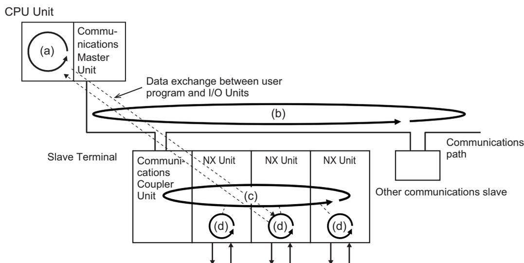
The cycle time of the CPU Unit, the communications cycle of the host network, and the NX bus I/O refresh cycle are determined by the model of the CPU Unit and the type of communications.
