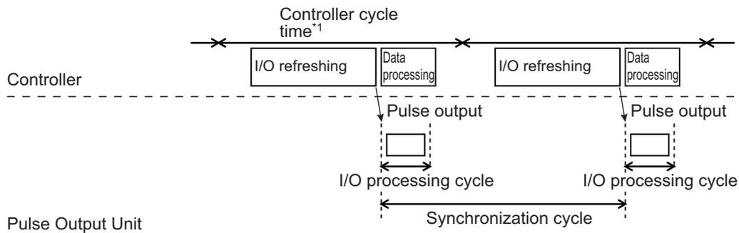
\*1. For an NX-series CPU Unit, the task period of the primary periodic task or priority-5 periodic task is applicable. For an NJ-series CPU Unit, only the task period of the primary periodic task is applicable.
