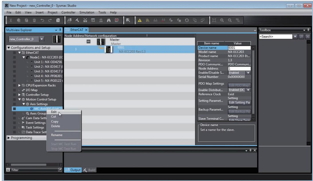
The Axis Basic Settings are displayed in the Axis Parameter Settings Tab Page.
