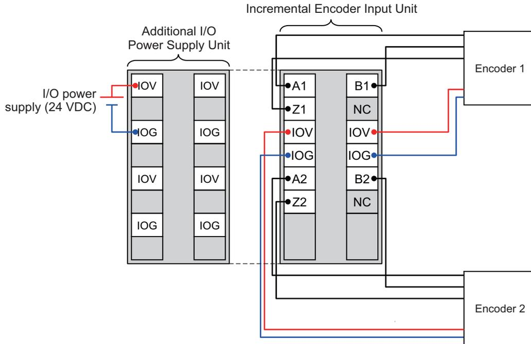
Note 1. The encoder inputs on Units with voltage inputs are NPN connections.
