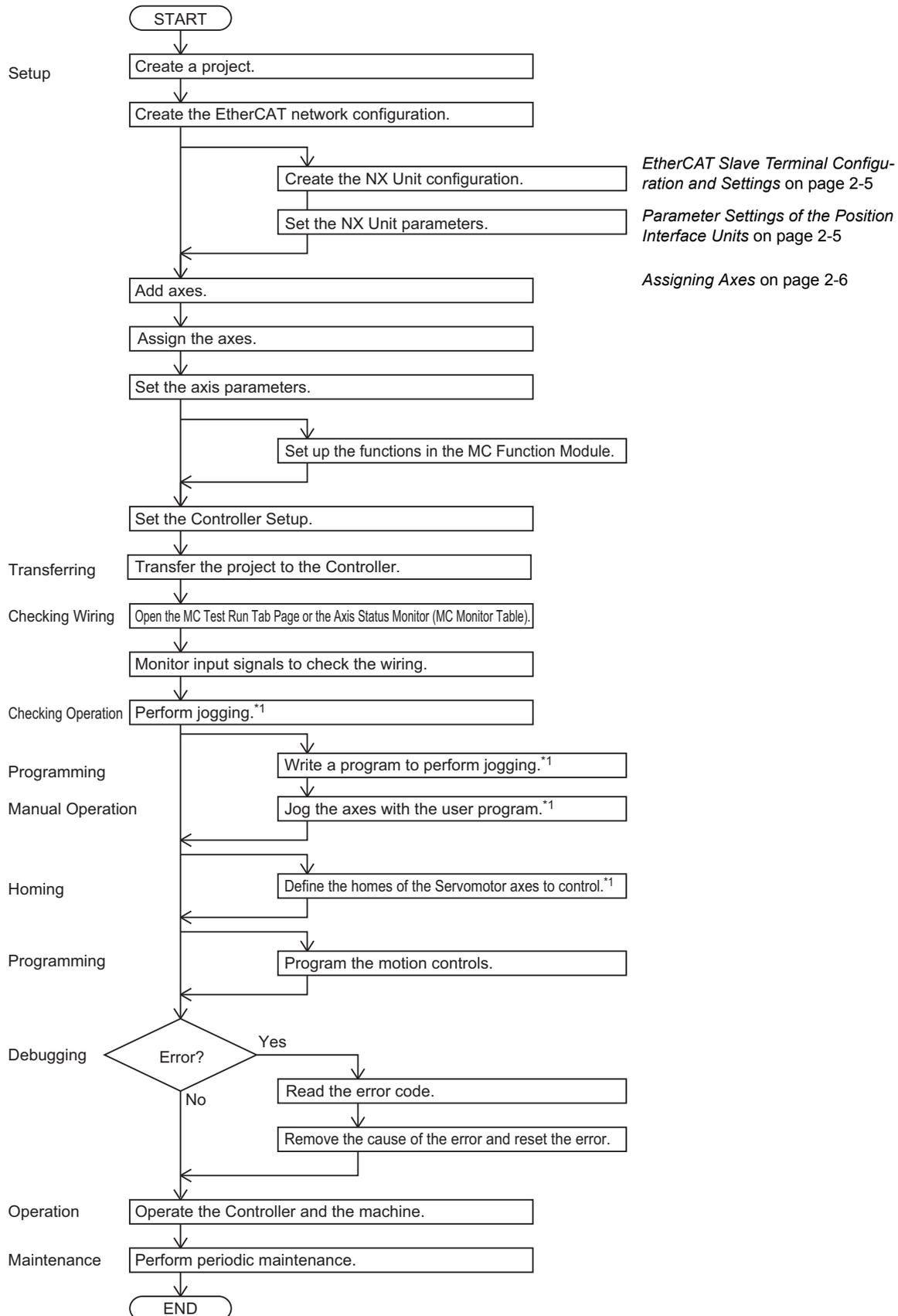
\*1. These steps are required if a Pulse Output Unit is used to control the motor drive.
