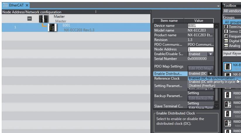
As a result, synchronous I/O refreshing is used.
