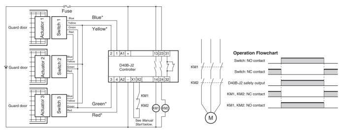
Note 1: The circuit in this example is equivalent to a Safety Category 3 circuit.
