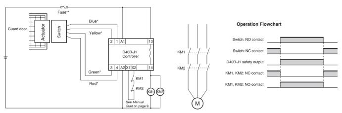
Note: The circuit in this example is equivalent to a Safety Category 3 circuit.
