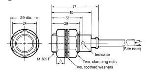
Oil-resistant, vibration-resistant, and fire-retardant, vinyl-insulated round cord, 6 dia., 0.5 dia. x 2 cores, standard length: 2 m Note: The cord can be extended in an independent conduit for 200 m maximum.
