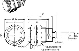
Oil-resistant, vibration-resistant, and fire-retardant, vinyl-insulated round cord, 6 dia., 0.5 dia. x 2 cores, standard length: 2 m  $\,$ The cord can be extended in an independent conduit for 200 m maximum.
