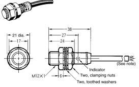
Note: Oil-resistant, vibration-resistant, and fire-retardant vinyl-insulated round cord, 6 dia., 0.5 dia. x 3 cores, standard length: 2 m The cord can be extended in an independent conduit for 200 m maximum.
