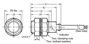
Note: Oil-resistant, vibration-resistant, and fire-retardant, vinyl-insulated round cord, 6 dia., 0.5 dia. x 3 cores, standard length: 2 m The cord can be extended in an independent conduit for 200 m maximum.
