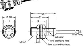
Oil-resistant, vibration-resistant, and fire-retardant, vinyl-insulated round cord, 6 dia., 0.5 dia. x 2 cores, standard length: 2 m  $\,$ Note: The cord can be extended in an independent conduit for 200 m maximum.
