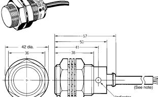
Oil-resistant, vibration-resistant, and fire-retardant, vinyl-insulated round cord, 6 dia., 0.5 dia. x 3 cores, standard length: 2 m  $\,$ Note: The cord can be extended in an independent conduit for 200 m maximum.
