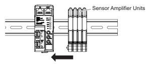
4. Use the DIN Track End Plates (PFP-M) that are provided to remove any gaps between the Units and secure them in place. Replace the protective cap that you removed in step 3 to the Sensor Amplifier on the right end.
