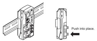
3. Remove the protective cap from the right side of the Sensor Communication Unit. Then, slide the Sensor Amplifier Units against the Sensor Communication Unit with the tabs aligned with the notches in the connector area. Press them together until they click into place.
