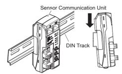
2. Press the lower portion of the Unit against the DIN Track.
