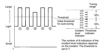
Taking into consideration the vibration of the sensing objects on the in-line operation, sample the incident with the first five sensing objects after setting the threshold and set the threshold again to the middle value between the highest and lowest incident values obtained with the sensing objects. The E3X-NH will then perform auto-tuning within a range of  $\pm 18\%$  of this value.
