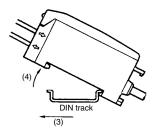
In the case of side mounting, attach the mounting bracket on the Amplifier first, and secure the Amplifier with M3 screws and washers. The diameter of the washers should be 6 mm max.
