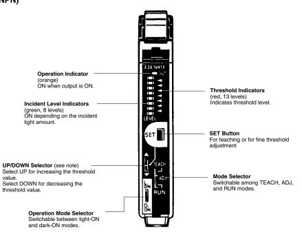
Note: Used for making fine-sensitivity adjustments.
