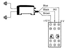
Note: A maximum of two E3X-NH Sensors can be connected.
