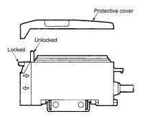
3. The fiber must be locked or released in a temperature range of  $-10^\circ C$  to  $40^\circ C.$
