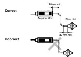
Do not apply excess force on the Fiber Units.
