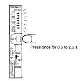
2. Set the mode selector to RUN. The threshold is set automatically.
