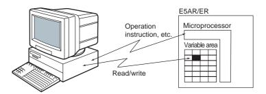
A variable area is accessed by specifying the position of a variable within the variable area using the variable type and address.
