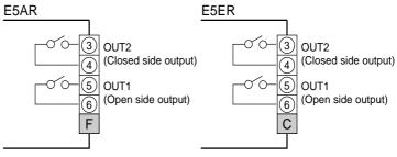
Relay output specifications are as follows: 250 V AC, 1 A (including inrush current)
