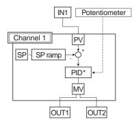
To control a gas kiln using a position proportional control valve, select the control valve control type and configure the instrumentation as shown in the following example.
