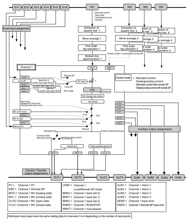
\* Cascade standard control, Cascade heating/cooling control, position proportional control and ratio control are also available. See "Section 3, Typical Control Examples" (page 3-1).
