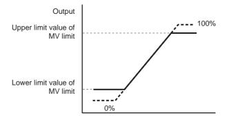
• In the case of heating/cooling control, overall upper and lower limits are set for heating and cooling. (Separate limit settings are not possible.)
