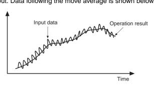
• This function is used to reduce changes in the input due to disturbances in the fluid surface when controlling fluid level.
