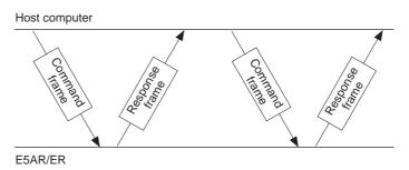
The exchange between the command frame and response frame is explained below.
