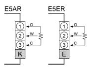
· For information on the potentiometer, see the manual for the valve you are connecting. Terminal number meanings are as follows. O:OPEN, W:WIPE, C:CLOSE The input range is 100  $\Omega$  to 2.5 k $\Omega$  (Between C to O).
