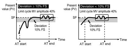
The amplitude of change of the limit cycle MV can be changed in "Limit cycle MV amplitude".
