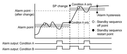
• After changing the standby sequence restart setting, a software reset must be executed or the power turned off and on to make the change take effect.
