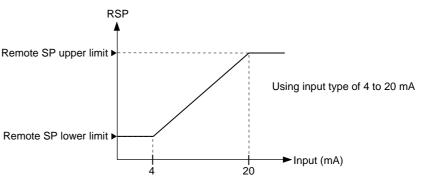
Note that the SP limits are in effect, and therefore if the input remote SP is above or below the SP limits, the SP will be clamped to the upper or lower limit.
