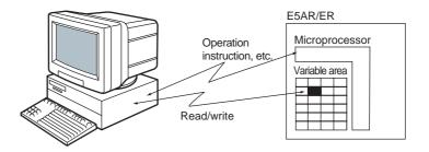
The variable area is accessed by specifying the position of a **variable** within the variable area using a channel identifier, area number, and in-area **address**.
