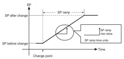
The rate of change during SP ramp is set in "SP ramp rise value", "SP ramp fall value", and "SP ramp time unit".
