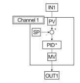
When controlling a heater plate for semiconductor wafers with the E5AR, the control mode is set to standard control and instrumentation is as shown in the following example.
