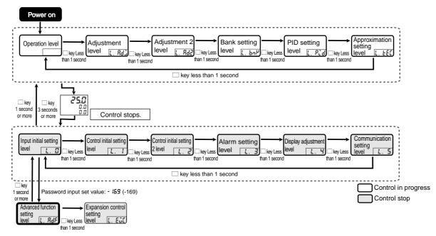
To move to Advanced function setting level, set "Initial setting level protect" in Protect level to "0", and then enter the password (-169) in "Move to Advanced function setting level" (Input initial setting level).
