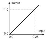
Straight-line approximation 2 is then used to convert this result from an industrial quantity to normalized data.
