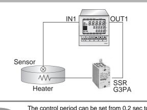
Hint The control period can be set from 0.2 sec to 99.0 seconds on the E5AR/ER. (The shortest setting on our previous models was 1 sec). For high precision control applications that previously required the combined use of our cycle control unit (G32A-EA) and an SSR, the G32A-EA is now no longer needed.
