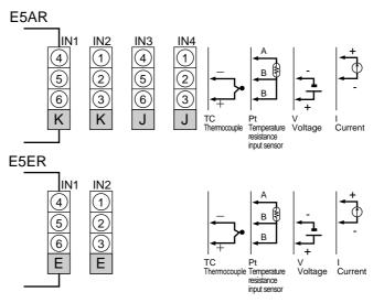
To prevent the appearance of error displays due to unused inputs, set the Number of enabled channels.
