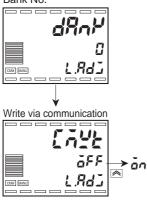
To allow a host computer to write setting data to a controller, set "Write via communication" (Adjustment level) to "an: Enabled".
