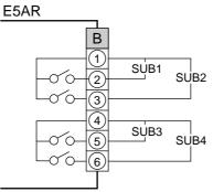
On the E5ER-□4□□, auxiliary outputs 1 to 4 (SUB1 to 4) output to terminals B1 to B6. On the E5ER-□T□□, auxiliary outputs 1 to 2 (SUB1 to 2) output to terminals D3 to D6.
