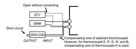
Disconnect the STV and enable the thermocouple in the cold junction compensator. Make sure that the STV is disconnected at this time.
