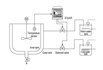
Hint In addition to control of chemical reactions and other processes that naturally generate heat, heating/cooling control is also being increasingly used to shorten heating and cooling cycles for improved production efficiency in batch process production. Example: Heating/cooling control of a flip chip bonding machine
