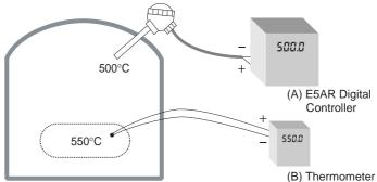
(Figure 1. Configuration for input shift)
