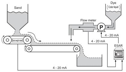
Settings are shown when 4 to 20 mA is used in the input from the dye flow sensor, 4 to 20 mA is used in the input from the sand weight measurement sensor, and a pump is used that is driven by an inverter with a 4 to 20 mA input is used in the manipulation system.
