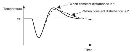
• The waveform may vary from that in the diagram depending on differences in the object of control and differences in PID values.
