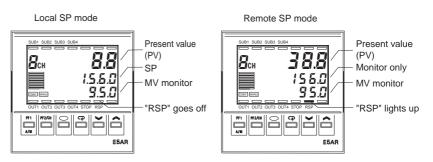
• When using a bank in local SP mode, a link is created to the local SP of the selected bank. For example, if Bank 3 is selected, the local SP of Bank 3 appears in Display 2, and when the value is changed, the value of "Bank 3 local SP" (Bank setting level) also changes.
