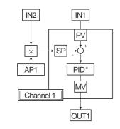
This machine mixes a constant proportion of flowing sand and dye in order to dye the sand a uniform color.
