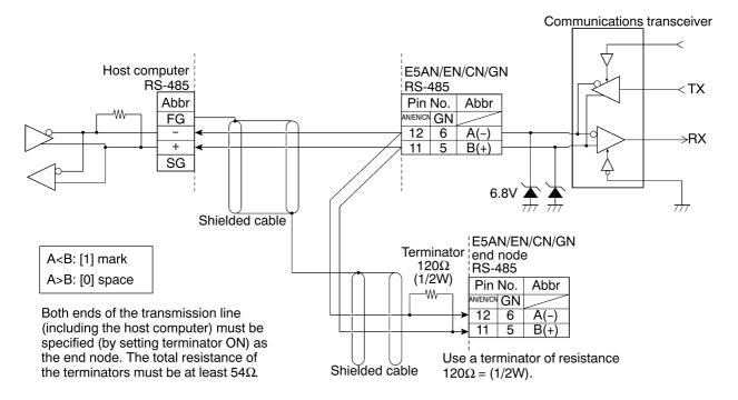
Match the communications specifications of the E5AN/EN/CN/GN and the host computer. If a one-to-N system is being used, be sure that the communications specifications of all devices in the system (except individual unit numbers) are the same.
