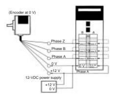
Note: Apply the following connections if the power supply to the E6C3 is 12 or 24 V.
