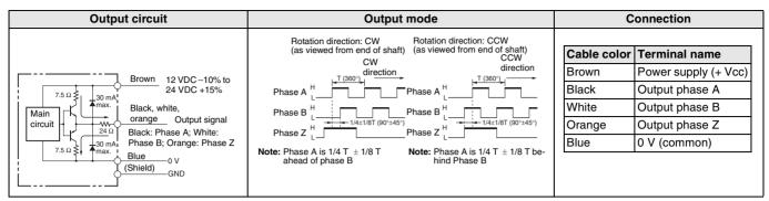
Note 1. The shielded cable outer core is not connected to the inner area or to the case.
