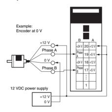
Note: When the encoder power supply is either 5 V or 24 V:
