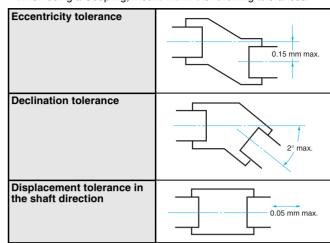
If the eccentricity or declination value exceeds the tolerance, an excessive load on the shaft may damage the E6F-C or shorten the life of the F6F-C.
