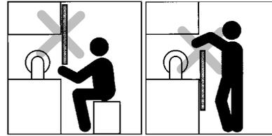
A worker is between the F3S-A detection zone and dangerous machine parts.
