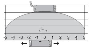
5 mm misalignment tolerance after setting
