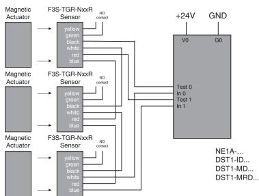
Application with multiple Sensors with NE1A or DST1-Safety-IO (up to Safety Category 4 acc. EN954-1)
