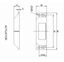
Small Sensor (Sensor/Actuator) F3S-TGR-NSMR
