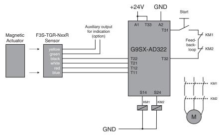
Series connection Application, up to 6 Sensors with G9SX-AD322-T15 (up to Safety Category 3 acc. EN954-1)
