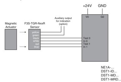
Series connection Application, up to 6 Sensors with NE1A or DST1-Safety-IO (up to Safety Category 3 acc. EN954-1)
