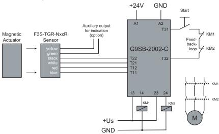
Series connection Application, up to 6 Sensors with G9SB-2002-C (up to safety Category 3 acc. EN954-1)
