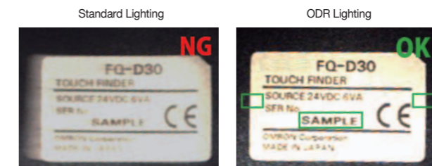
Inspection is not possible because of workpiece blurring or a lack of brightness.
