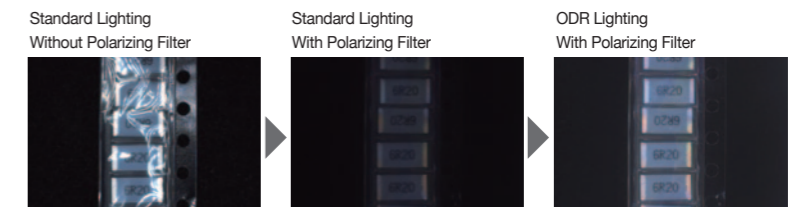
It is impossible to detect the workpiece because of reflections from the film.
