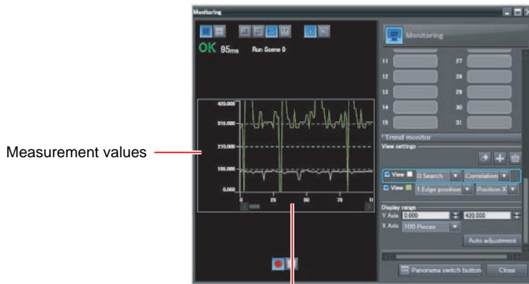
Changes in the measured values of the selected inspection item are displayed against time in a graph.
