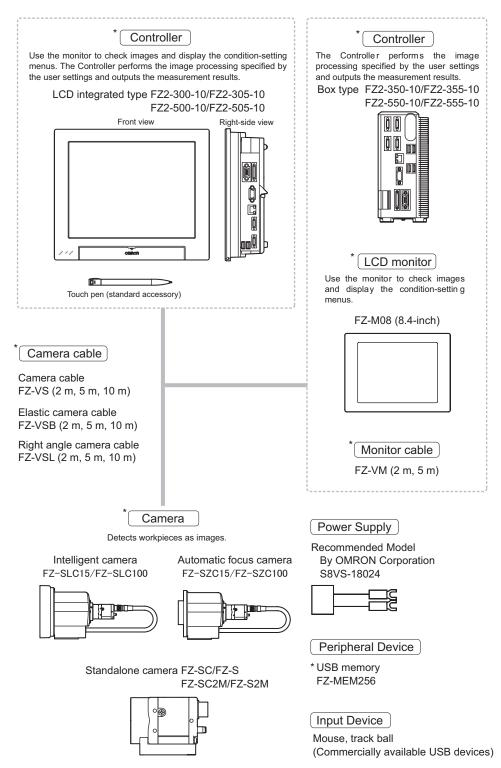
\*FZ-SC2M/FZ-S2M camera can be connected only with FZ2-50\_-10/FZ2-55\_-10 controller.
