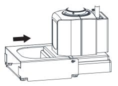
Rotate the mounting brackets to secure the FZ-SLC15 illumination with the provided hexagonal wrench.
