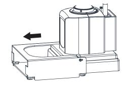
Securely tighten the screws of the mounting brackets with the provided hexagonal wrench.
