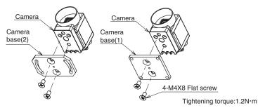
②Set up the camera bases on the each predefined position with pan screws M3X8 (accessory).
