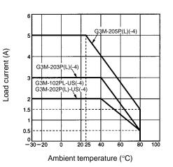
Non-repetitive Reduce the current to 1/2 or less if the G3M is in repetitive operation.
