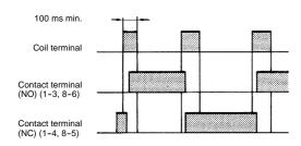
Note: When a pulse for application to the coil is used, such a pulse should have a width of 100 ms or more. If a pulse is applied with a width less than the operate time, the cam may fail to rotate fully.
