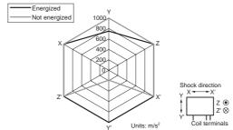
Measurement conditions: Impose a shock in the  $\pm X$ ,  $\pm Y$ , and ±Z directions three times each with the Relay energized to check the shock values that cause the Relay to malfunction.
