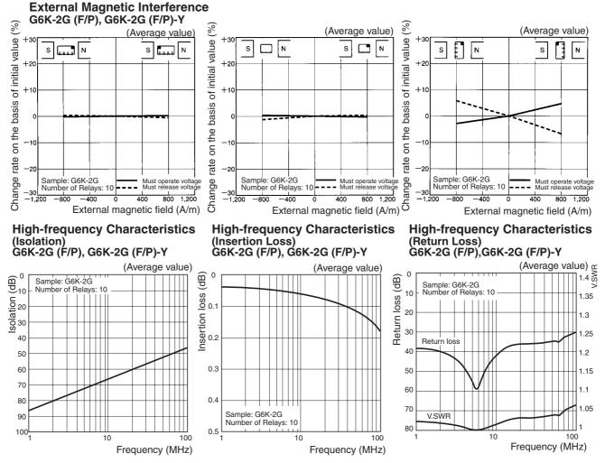
Note: 1. The tests were conducted at an ambient temperature of 23°C.
