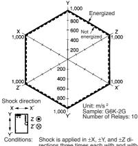
Shock is applied in ±X, ±Y, and ±Z directions three times each with and without energizing the Relays to check the number of contact malfunctions.
