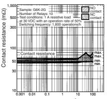
Operating frequency (x10<sup>3</sup> operations) **Note:** The tests were conducted at an ambient temperature of 23°C.
