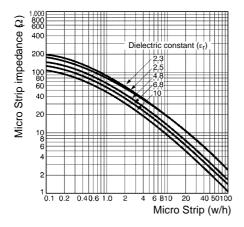
For example, when creating 50-Ω lines using a glass epoxy base with a thickness of 1.6 mm, the above graph will yield a w/h ratio of 1.7 for a dielectric constant of 4.8. Since the base thickness is 1.6 mm, the width will be h x 1.7 ≈ 2.7 mm.
