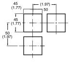
Note: Recommended panel thickness is 1 to 3.2 mm.
