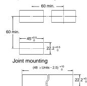
Waterproofing is not possible for joint mounting
