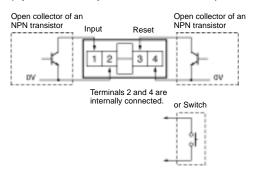
Note: 1. Residual voltage in the output section of Proximity Sensors or Photoelectric Sensors becomes less than 0.5 V because the current flowing from terminals 1 or 3 is as small as approx. 10 μA, allowing easy connection.
