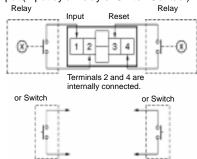
Note: Use Relays and Switches that have high contact reliability because the current flowing from terminals 1 or 3 is as small as approx. 10 μA. OMRON's G3TA-IA/ID is recommended as the SSR.
