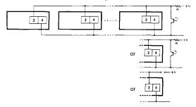
Note: H (Reset ON) level must be 4.5 V minimum. H =  $\frac{4.7 (k\Omega)/N + V}{M}$
