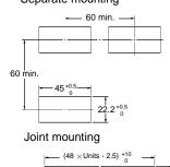
Waterproofing is not possible for joint mounting
