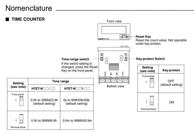
Note: Perform switch setting before mounting to a control panel.
