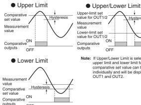
Note: If Upper/Lower Limit is selected, the upper limit and lower limit for the comparative set value can be set individually and will be displayed for
