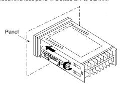
Attach the mounting bracket on the left and right sides of the Intelligent Signal Processor as shown in the illustration above and gradually tighten each screw evenly in turn by considering the balance of the tightening force until the ratchets start slipping without being further tightened.
