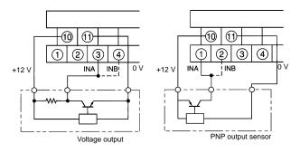
When inputting the external control signals through the open collector:
