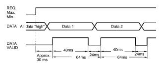
The K3NP outputs each measurement at an interval of 64 ms when a REQ signal is ON continuously.
