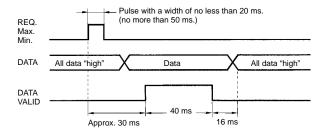
Approximately 30 ms after the REQ signal rises, a sample is taken and the DATA VALID signal is output. Read the data when the DATA VALID signal is ON.
