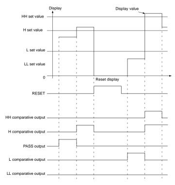
Note: Because measuring is not continuous, the comparative output turns ON when the measuring operation is completed.
