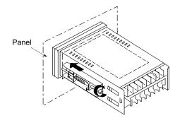
Attach the mounting bracket on the left and right sides of the Intelligent Signal Processor as shown in the illustration above and gradually tighten each screw evenly in turn by considering the balance of the tightening force until the ratchets start slipping without being further tightened.
